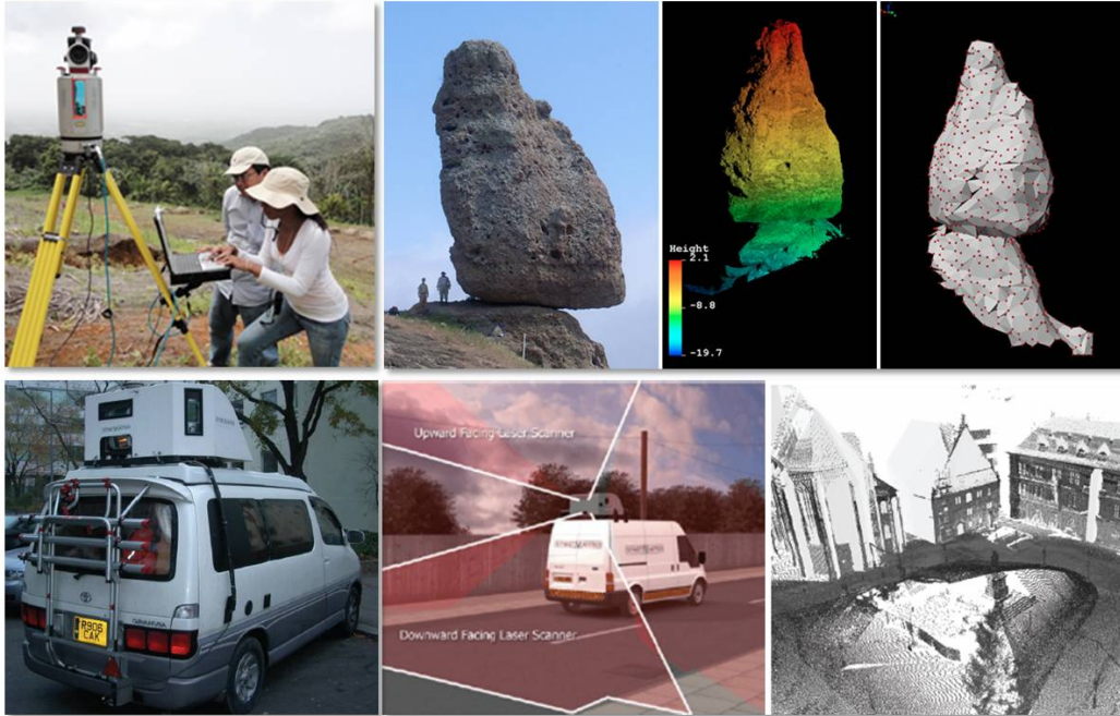
Figure 1.6: Top-left: Image of Terrestrial Laser Scanner (Riegl VZ-400) mounted on a tripod and operated by Professor Guoquan Wang and student Arlenys Ramiriz from the University of Puerto Rico at Mayaguez. Top-right: the resulting Lidar data and modeling. The images are courtesy of the UNAVCO project [UNAVCO 2008]. Bottom-left: Image of StreetMapper mobile laser scanning system. Bottom-right: the resulting Lidar data. Images courtesy of [Haala 2008].
