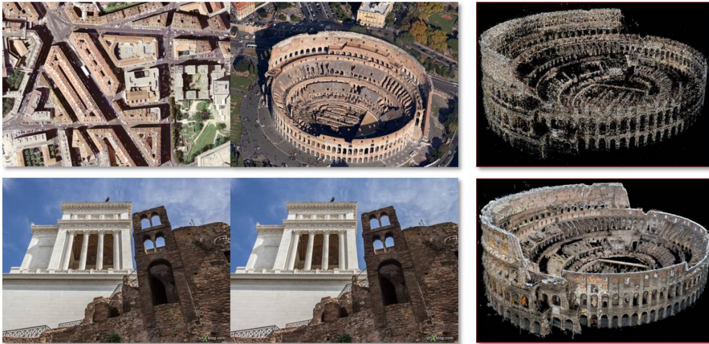
Figure 1.2: Illustration of image data with corresponding scene reconstruction. Top-left: Examples of aerial image data. Bottom-left: Examples of stereo ground-based image data. Top-right: Reconstruction of the coliseum by Structure from Motion (SfM) technique with images from Flickr. Bottom-right: Reconstruction of the coliseum by patch of Multi-View Stereo (MVS) technique with images from Flickr. Both SfM and MVS images courtesy of Furukawa et al. [Furukawa 2010].
