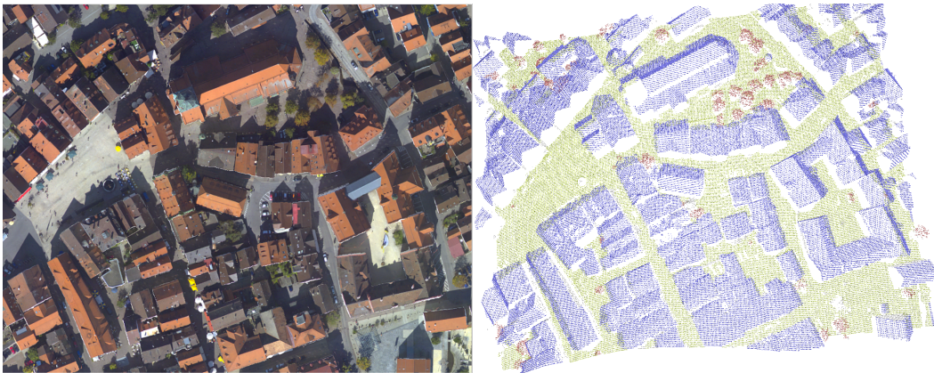
Figure 2.2: Point cloud classification- An aerial image ( left ) and the classified point set ( right ). Note that the four classes building (in blue), vegetation (in red), ground (in green), and NC (in white) are correctly separated. Images courtesy of Google [Google 2013].
