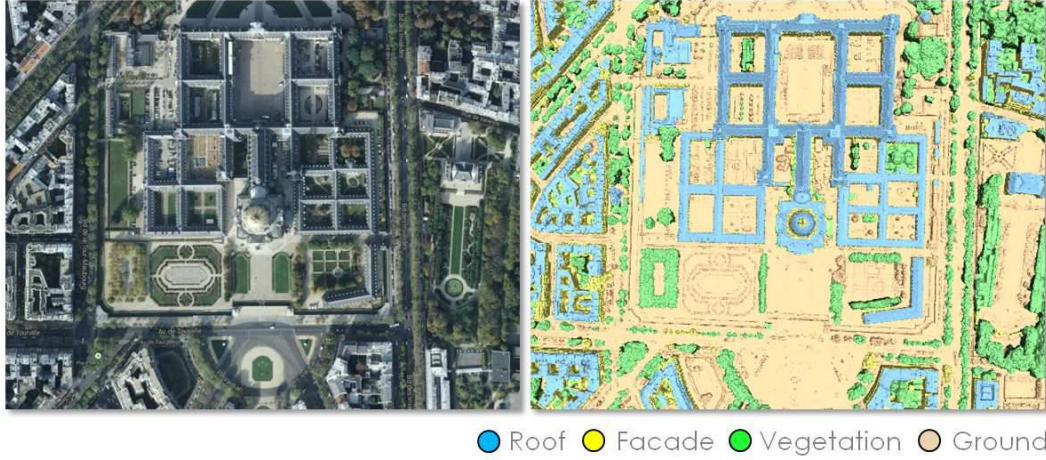
Figure 2.4: MVS classification- An aerial image ( left ) and the classified MVS data ( right ). Note that the four classes building , vegetation , ground , and facade are correctly separated. Image courtesy of Google [Google 2013].
