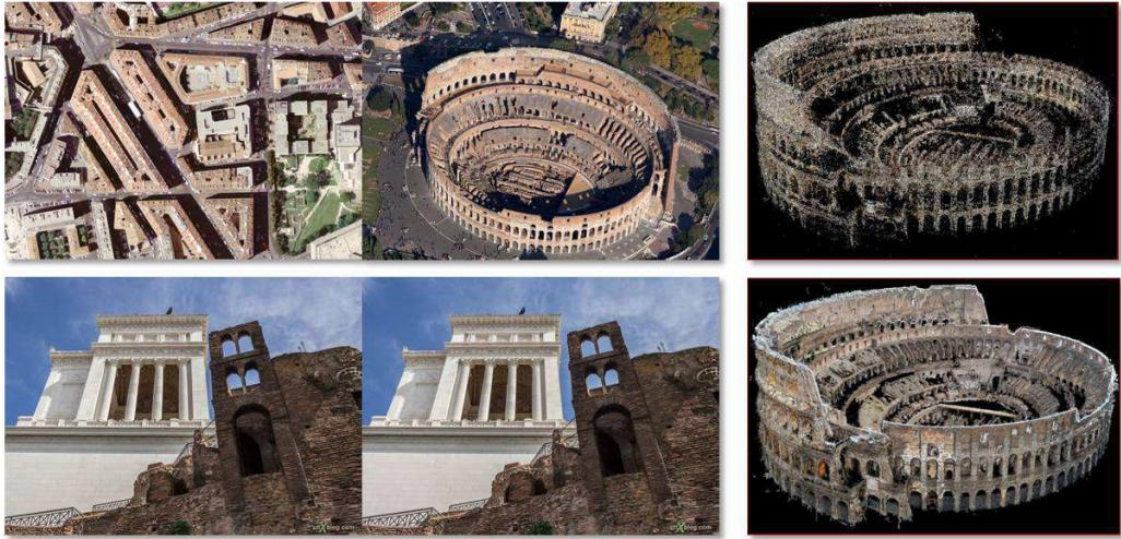
Figure 1.2: Illustration of image data with corresponding scene reconstruction. Top-left: Examples of aerial image data. Bottom-left: Examples of stereo ground-based image data. Top-right: Reconstruction of the coliseum by Structure from Motion (SfM) technique with images from Flickr. Bottom-right: Reconstruction of the coliseum by patch of Multi-View Stereo (MVS) technique with images from Flickr. Both SfM and MVS images courtesy of Furukawa et al. [Furukawa 2010].
