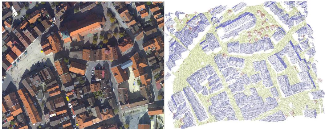
Figure 2.2: Point cloud classification- An aerial image (*left*) and the classified point set (*right*). Note that the four classes *building* (in blue), *vegetation* (in red), *ground* (in green), and *NC* (in white) are correctly separated. Images courtesy of *Google* [Google 2013].
