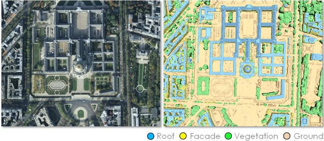
Figure 2.4: MVS classification- An aerial image (*left*) and the classified MVS data (*right*). Note that the four classes *building*, *vegetation*, *ground*, and *facade* are correctly separated. Image courtesy of Google [Google 2013].
