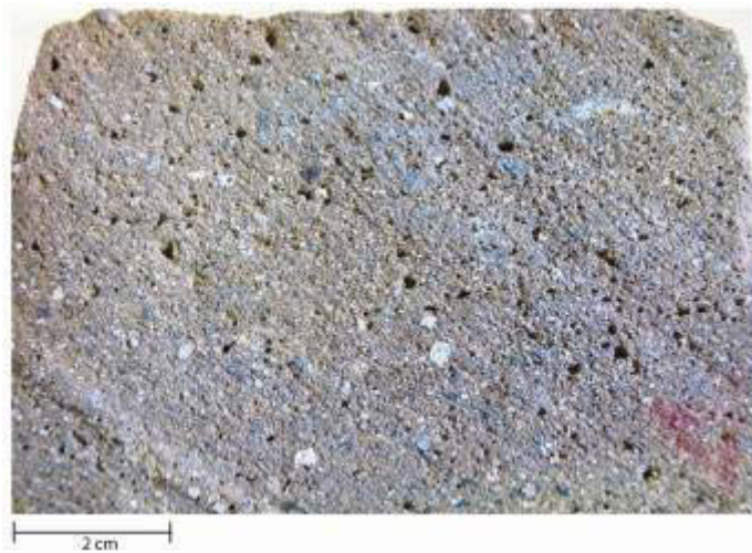
Figure 4.17: Red clay brick sourced from handmade brick factory in Quebrada Huarangal, Arequipa.
