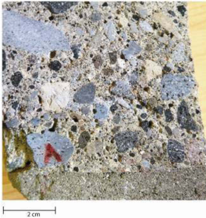
Figure 4.19: Concrete block sourced from a disused building in Arequipa. Note the concrete stucco facing to the bottom of the image.
