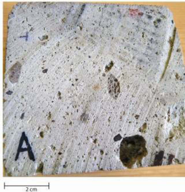
Figure 4.18: Ignimbrite block sourced from a brick factory in Arequipa.
