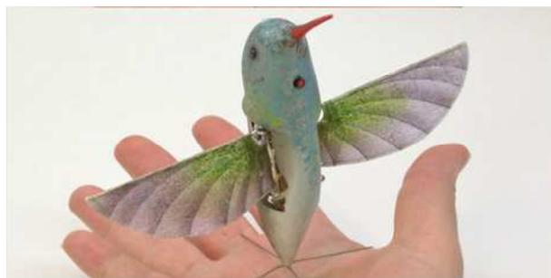
FIGURE 1.4 – Exemple de micro-drone à voilure battante (Hummingbird, AeroVironment).
