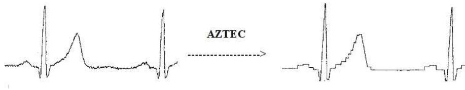
Figure III.4: Algorithme de compression AZTEC[83]
