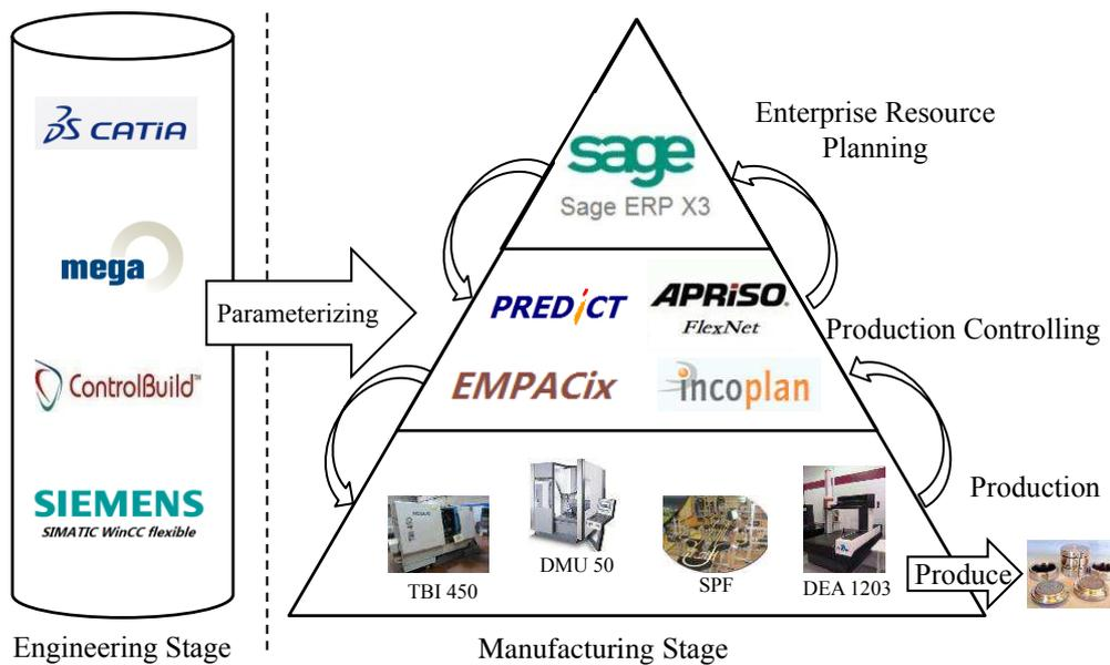
Figure 5-1 The System Stack in the AIPL
