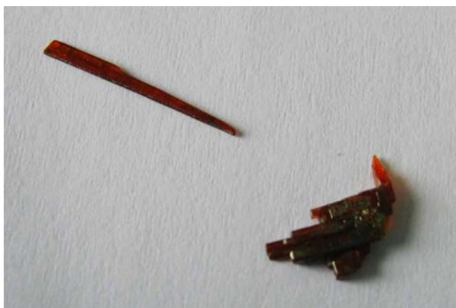
FIGURE 2.27: Photo of the PEPI crystal bulks grown from nitromethane/acetone mixed solution.
