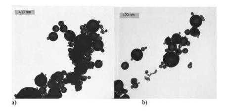
FIGURE 2.32: TEM pictures of the nanoparticles (a) AMPI and (b) CMPB. The hollow character of large particles is quite apparent in (b). Audebert et al. (2009)
