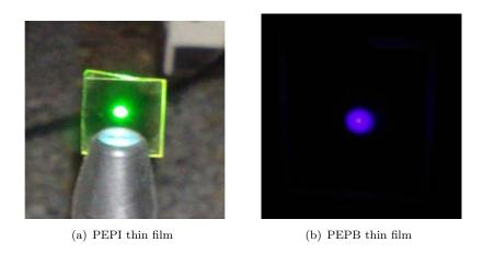
Figure 2.7: Photoluminescence of thin films of several tens nm (a) PEPI (the excitation wavelength is 405 nm, diode laser), (b) PEPB (the excitation wavelength is 325 nm , HeCd laser.
