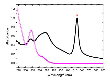
FIGURE 2.16: OA spectra of a 50 nm PEPI thin film (black line) and of a solution containing PEPI dissolved in DMF solvent (pink line).
