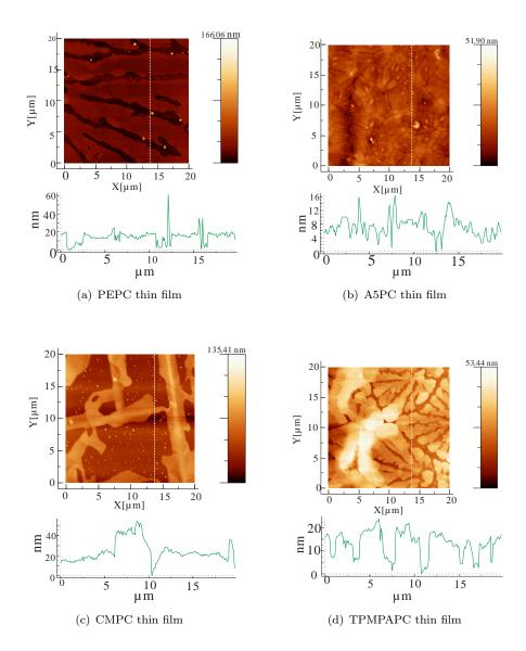
FIGURE 3.7: AFM images of PEPC, A5PC, CMPC and TPMPAPC thin films. The vertical cross-sections marked with white dotted lines in (a), (b), (c) and (d) are presented in graphs below, for each perovskite thin film.
