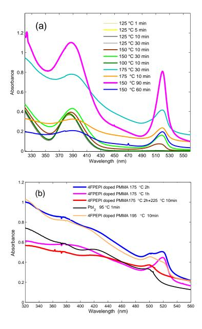
FIGURE 4.28: Comparative absorbance of 4FPEPI doped PMMA layers made from 20 wt% solutions. These samples are annealed at different temperature, and exhibit different absorption intensities, as seen in (a). (b) The 4FPEPI doped PMMA layers annealed at over high temperature condition. Measurement is carried on at room temperature.
