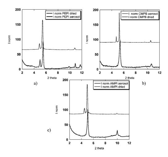
Figure 2.33: X-Ray diffraction spectra of the (a) PEPI, (b) CMPB, and (c) AMPI perovskites. The full lines correspond to the spectra of the nanoparticles and the dotted lines to the spectra of a bulk sample dried in the air.
