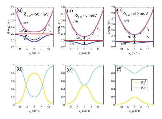
FIGURE 5.7: Dispersion curves of UPB and LPB and Hopfield coefficients for three different detunings: (a), (d)  $\delta_{p-ex} = -50$  meV; (b), (e)  $\delta_{p-ex} = 0$  meV and (c), (f)  $\delta_{p-ex} = 50$  meV.
