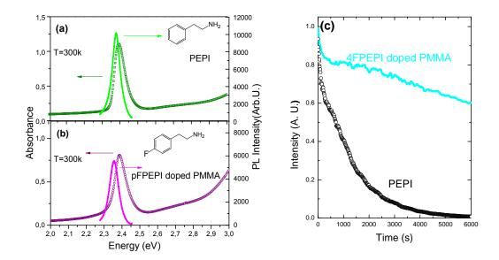
FIGURE 5.24: Optical density (scatters) and photoluminescences spectra (solid lines), at T = 300 K, of (a) a 50 nm PEPI thin layer , (b) a 1  $\mu$ m 4FPEPI doped PMMA thin layer.(c) Photobleaching of 4FPEPI doped PMMA and PEPI thin layers under the laser HeCd 325nm for 6000 s.
