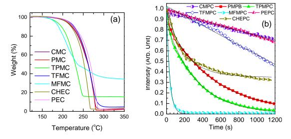
FIGURE 4.2: (a) Thermogravimetric measurements of organic salts, and (b) evolution of PL intensity versus time for the UV  $(T-(CH_2)_nNH_3)_2PbCl_4$  perovskites. The measurements are performed in air at room temperature. PL is excited at 325 nm with a HeCd laser with incident power of 18 mW.
