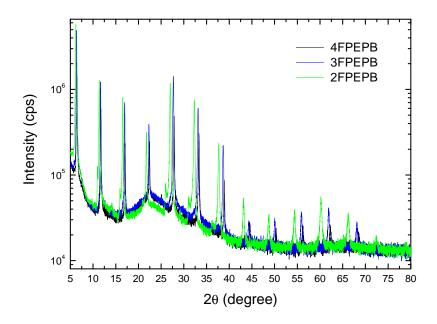
FIGURE 4.20: X-ray diffraction spectra of 4FPEPB, 3FPEPB and 2FPEPB spin-coated layers
