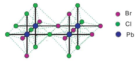
FIGURE 3.15: Schema of  $PbCl_xBr_{4-x}^{2-}$  mixed wells. The Br and Cl atoms are distributed in a randomized way inside the inorganic layers.
