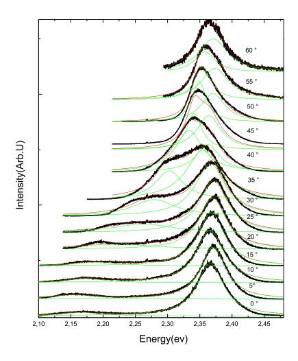
FIGURE 5.27: PL spectra of 4FPEPI doped PMMA cavity. PL signals are detected from 0° to 60°. Each PL curve is fitted by two lorentzian peaks(in green), and the red curve is a sum of the two lorentzian peaks.
