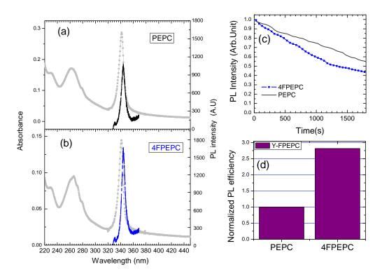
FIGURE 4.23: Comparative (a) absorption, (b) photoluminescence and (c) photobleaching rate of PEPC and 4FPEPC layers, made from 1.5wt% solutions. The excitation laser is the 325 nm line HeCd laser. For the PL, the excitation laser power is 2 mW, it is 7 mW for the bleaching rate. (d) Normalized PL efficiency of these perovskites layers.
