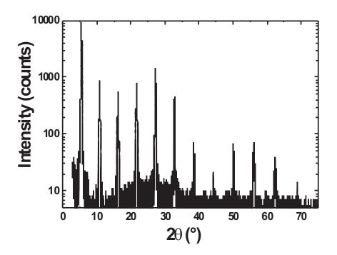
FIGURE 2.1: XRD spectrum of a 50 nm PEPI thin film, performed at LPN Marcoussis. Gauthron et al. (2010)
