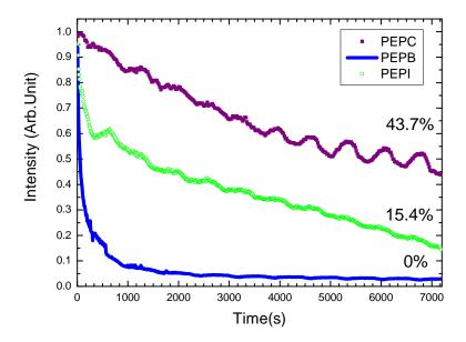
FIGURE 4.8: PL intensity as a function of illumination time for PEPI, PEPB and PEPC thin films in He environment. Laser power is 7 mW (325 nm line).
