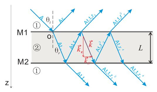
Figure 5.1: Geometry of a simple planar cavity
