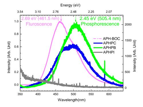
FIGURE 5.37: PL spectra of APH-BOC and APHPX (X = Cl, Br and I) film samples.
