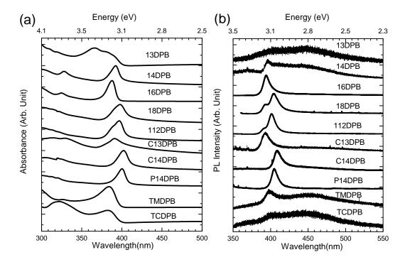
FIGURE 3.8: (a) OA and (b) PL of some lead bromide diammoniums based 2D layered perovskites. PL curves are normalized. The curves are displaced vertically for clarity. The experiments are carried on at room temperature and the excitation source for PL is the 325 nm line of a HeCd laser, the power is 1 mW.
