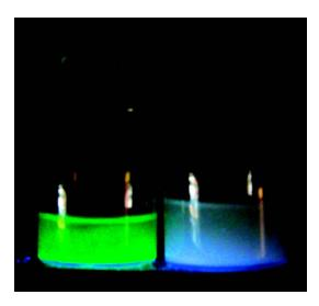
FIGURE 2.31: Luminescence, under UV lamp, of the nanoparticles dispersed in hexane: left, PEPI; right, CMPB.
