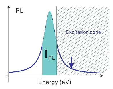
FIGURE 2.9: Principle of PLE (Excitation of the photoluminescence) measurement
