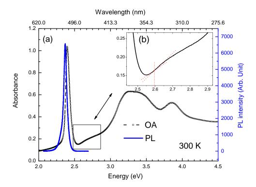
FIGURE 2.22: (a) OA spectrum and PL spectrum of a 50 nm thick PEPI film measured at room temperature. The excitation source for PL measurement is the 325 nm line of a HeCd laser, with an incident power of 0.6 mW. The insert graph (b) is a zoom of the square zone in graph (a) in order to show the step-like structure in OA spectrum.
