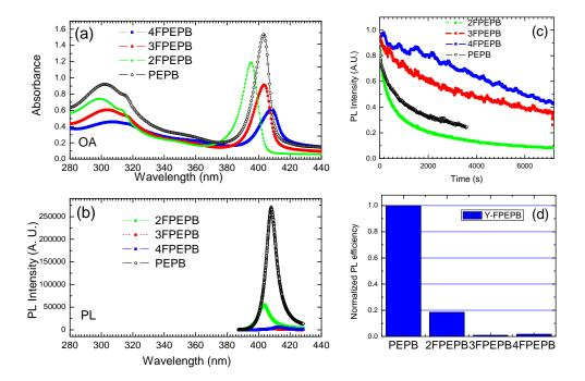
FIGURE 4.21: Comparative (a) absorbance, (b) photoluminescence and (c) photobleaching rate of bromide based perovskite layers made from 10wt% solutions. The excitation laser is the 325 nm line HeCd laser. For the PL and bleaching rate, the power is 1 mW. (d) Normalized PL efficiency of these perovskites layers.
