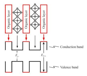
FIGURE 1.4: Schematic electronic structure of 2D layered organic-inorganic perovskites. The thickness of inorganic and organic layers are around 0.6 nm and 1 nm respectively. The HOMO-LUMO energy gap  $\mathbf{E}_{H-L}$  of organic barriers is larger than the energy gap of inorganic wells  $\mathbf{E}_q$ . Mitzi et al. (2001b)
