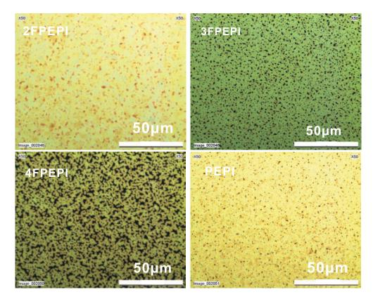
Figure 4.17: Optical microscope pictures of different perovskite layers prepared from 10% solutions.
