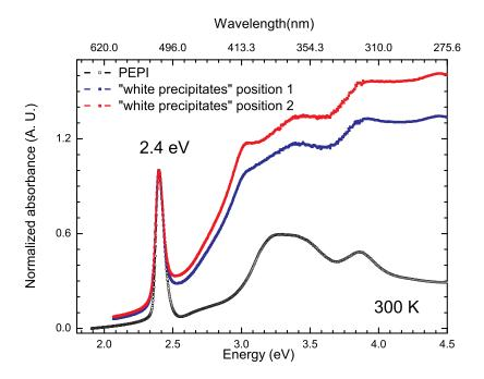
FIGURE 2.26: OA spectra of PEPI thin films deposited from the "white precipitates" in DMF solution as explained in the text. The black curve is the absorption spectrum of a 50 nm PEPI thin film prepared in conventional ways.
