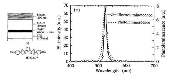
FIGURE 1.10: Device structure of an organic-inorganic heterostructure EL device using a PEPI spin-coated film (a) and molecular structure of an oxadiazole derivative OXD7 (in the scheme (a), PAPI states for PEPI) (b). Electroluminescence spectrum of an organic-inorganic heterostructure device using a PEPI spin-coated film at liquid-nitrogen temperature (c). The dotted line shows photoluminescence spectrum of a PEPI spin-coated film. Era et al. (1994)
