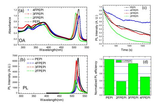
FIGURE 4.22: Comparative (a) absorbance, (b) photoluminescence and (c) photobleaching rate of iodide based perovskite layers made from 10wt% solutions. The excitation laser is the 325 nm line HeCd laser. For the PL, the excitation laser power is 0.6 mW, for the bleaching rate, it is 7 mW. (d) Normalized PL efficiency of these perovskites layers
