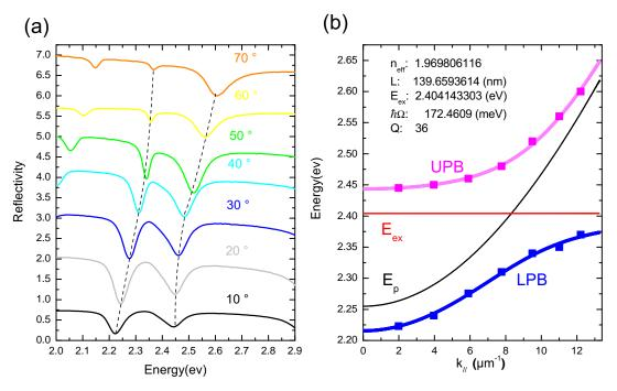
FIGURE 5.16: (a) Reflectivity spectra and (b) dispersion curve of a PEPI cavity with anticrossing around  $k_{//}=8.3~\mu\mathrm{m}^{-1}$  (detuning  $\delta_{p-ex}=$  -147 meV). The dashed line across dips in (a) are guides for the eyes and the reflectivity curves are displaced along y axis for clarity
