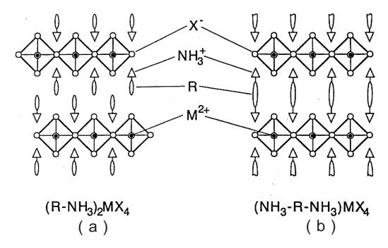
Figure 1.2: 2D-layered perovskites with (a) organic monoammonium cations and (b) diammonium cations. Mitzi (1999b)
