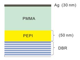
FIGURE 5.13: Schema of structure of a "standard cavity" PEPI microcavity.
