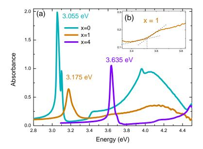
FIGURE 3.17: (a) OA spectra measured at 10 K in He environment for  $PEPC_xB_{4-x}$  mixed perovskites with x=0, 1 and 4. The insert graph (b) is a zoom of x = 1 case, in order to see clearly the step-like structure.
