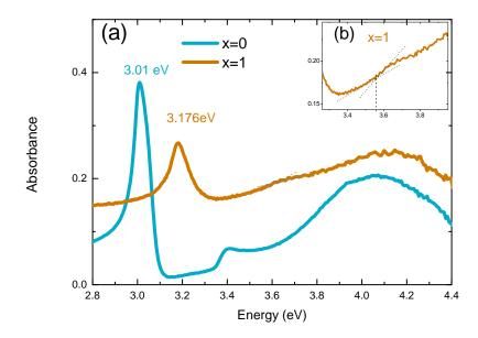
FIGURE 3.18: (a) OA spectra measured at 10 K in He environment for CMPB and  $CMPC_1B_3$  perovskites. The insert graph (b) is a zoom of x=1 case, in order to see clearly the step-like structure.
