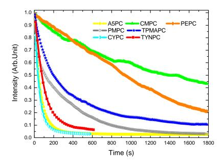
FIGURE 4.9: Photobleaching curves for PEPC, PMPC, CMPC, A5PC, TPMAPC, TNYPC and CYPC in air. The laser power is 7 mW at 325 nm.
