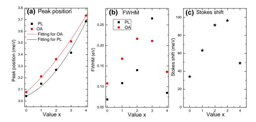
FIGURE 3.16: (a) OA and PL peak positions, (b) FWHM, and (c) Stokes-shift for  $CMPC_xB_{4-x}$  mixed perovskites. Data informations are extracted from OA and PL spectra in Figure 3.14. Parameters used for the fits are indicated in the text.
