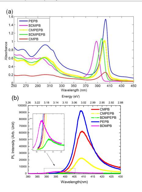
FIGURE 3.26: Optical spectra measured at room temperature: (a) OA spectra (b) PL spectra for PEPB, BDMPB, CMPB, BDMPEPB and CMPEPB thin films. The laser used as excitation is the 325 nm line of HeCd laser, the power is fixed at 5 mW.
