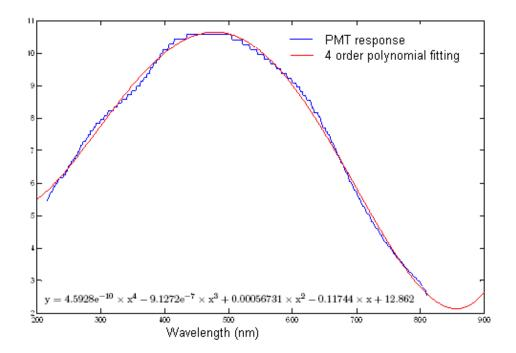
FIGURE 2.11: PMT response curve of the H9307-03 type PMT; the red curve is 4 order polynomial fitting curve
