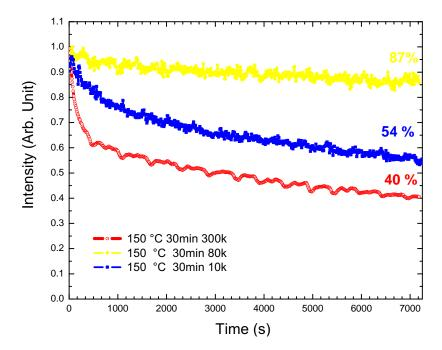
FIGURE 4.33: Photobleaching of 4FPEPI doped PMMA thin layer under the 325 nm line of a HeCd laser during 7200 s, the excitation power is kept at 7 mW. The measurement is carried on at room temperature. The thickness of 4FPEPI doped PMMA layer is around 1  $\mu$ m.
