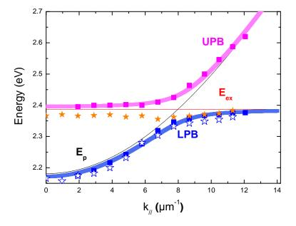
FIGURE 5.26: Polariton dispersion (LPB and UPB) measured from reflectivity spectra of Figure 5.25. Uncoupled perovskite exciton  $E_{ex}$  and cavity photon  $E_p$  are also shown. The stars represent the energy position of the PL peaks observed in Figure 5.27.
