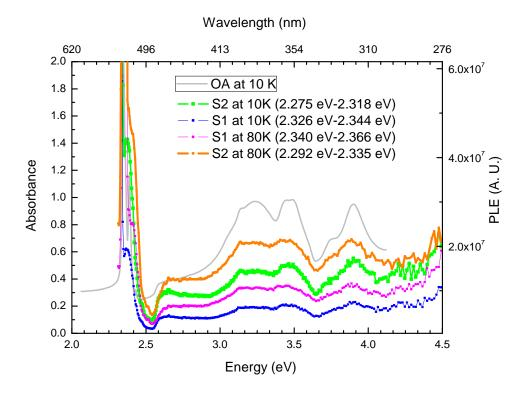
FIGURE 2.25: PLE spectra of S1 and S2 PL peaks (observed in Figure 2.24) of a 50 nm PEPI thin film at 10 K and 80 K. The grey curve is absorption spectrum measured at 10 K. The energy interval between brackets is the energy interval on which the PL intensity of S1 and S2 peaks are calculated.
