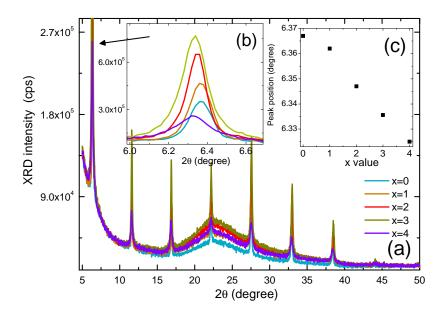
FIGURE 3.12: (a) X-ray Diffraction pattern for  $\mathrm{CMPC}_x\mathrm{B}_{4-x}$  mixed perovskites fabricated on quartz substrate. The solutions used for deposition are 0.026 mol/L. The insert graph (b) is the a zoom of the first peak around 6.35 °. The insert graph (c) shows the evolution of the peak position of the first mode versus x value.
