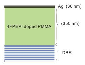
FIGURE 5.21: Schema of structure of a 4FPEPI doped PMMA microcavity.
