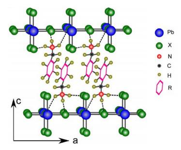
FIGURE 1.3: Sketch of 2D organic-inorganic lead halide semiconductors  $(R-NH_3)_2MX_4$ . The  $R-NH_3^+$  head binds to the inorganic sheet by two terminal halogens and one bridging halogen.
