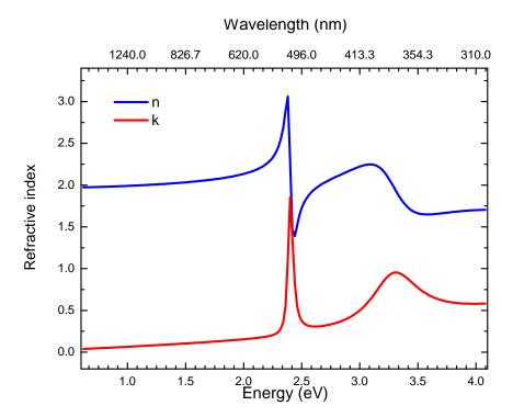
FIGURE 2.15: Refractive index  $\tilde{n} = n + i\kappa$  of PEPI film obtained from the fitting of  $\tan \psi$  and  $\cos \Delta$  in Figure 2.13. The blue curve and red curve represent the real n and imaginary  $\kappa$  parts of the refractive index respectively.
