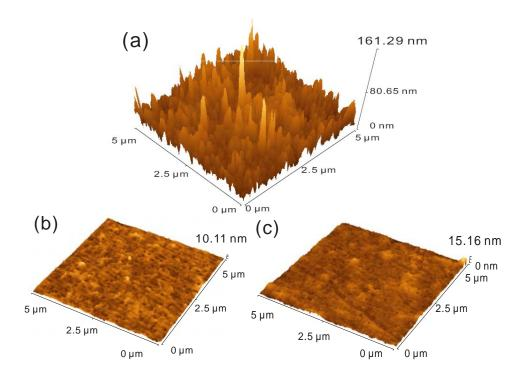
FIGURE 4.26: AFM images of (a) a 50 nm PEPI layer, (b) a 1  $\mu$ m 4FPEPI doped PMMA layer and (c) a 1  $\mu$ m PEPI doped PMMA layer. Be careful that the vertical scales are different in these two images
