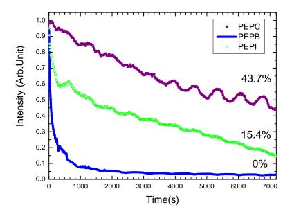
FIGURE 2.8: PL intensity as a function of illumination time for PEPI, PEPB and PEPC thin films in He environment. Laser power is 7 mW (325 nm line).
