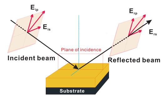
Figure 2.12: Principle of ellipsometry measurement
