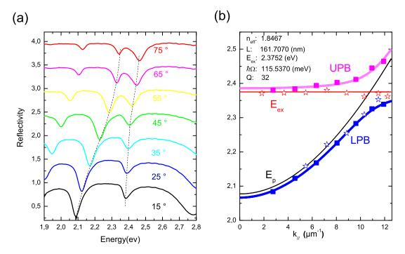
FIGURE 5.18: (a) Reflectivity and (b) dispersion curve of a PEPI cavity with anticrossing around  $k_{//}=10.7~\mu m^{-1}$  (detuning  $\delta_{p-ex}=$  - 298 meV). The dashed line across dips in (a) are guides of eyes and the reflectivity curves are displaced along y axis for clarity. The stars correspond to PL peak positions from angle resolved PL measurements of Figure 5.19.
