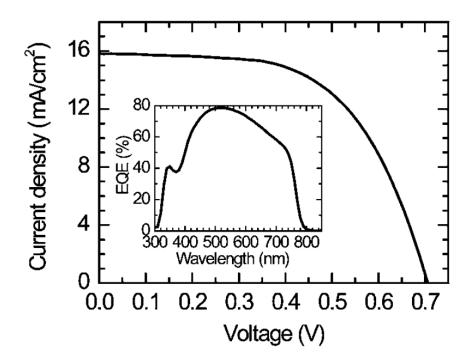
FIGURE 1.12: Photocurrent-voltage curve and EQE (External Quantum Efficiency) for the perovskite (CH<sub>3</sub>NH<sub>3</sub>)PbI<sub>3</sub> QD-sensitized  $TiO_2$  film whose surface was modified with Pb(NO<sub>3</sub>)<sub>2</sub>. Thickness of  $TiO_2$  film was 3.6 mm and the redox electrolyte used was composed of 0.9 M LiI, 0.45 M I<sub>2</sub>, 0.5 M tert-butylpyridine and 0.05 M urea in ethyl acetate. Koutselas et al. (2011)
