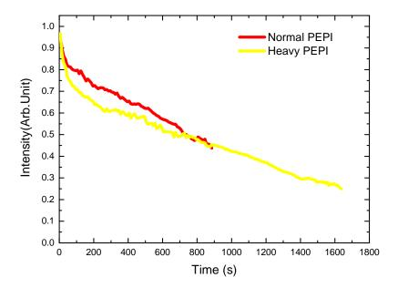
FIGURE 4.5: Evolution of PL intensity as a function of illumination time for normal PEPI (red line) and heavy PEPI (yellow line). The laser power is 7 mW at 325 nm.
