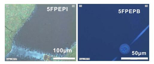
FIGURE 4.19: Spin-coated layers of 5FPEPI and 5FPEPB. The dewetting of the solution is shown, and the deposit lets appear inhomogeneous areas.
