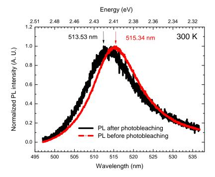
FIGURE 4.13: PL spectra of 2FPEPI before (in red) and after (in black) photobleaching. The measurement is carried on in air at room temperature, the laser power is 7 mW at 325 nm. PL intensities are normalized to 1.
