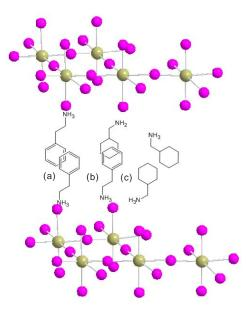
FIGURE 3.29: Sketch of a possible structure of CMPEPB. The mixed organic layer is composed with two organic ammoniums (CM and PE salts) stacking one with another via interaction among molecules: (a)  $\pi - \pi$ , (b) Van der Waals or (c) hydrogen bond.
