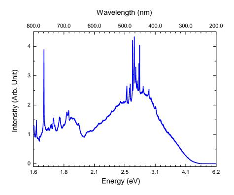
Figure 2.4: Emission spectra of Xenon lamp, the intensity is corrected by the response of the PMT detector.
