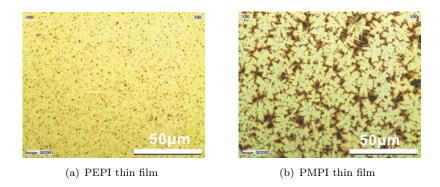
FIGURE 3.5: Images under microscope for (a) a PEPI thin film and (b) a PMPI thin film
