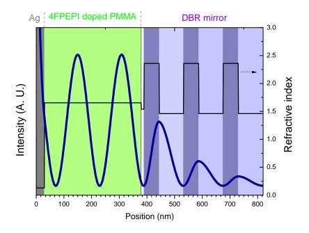
Figure 5.23: Profile of the electric field for the cavity mode energy 2.4 eV (blue line). The black line presents the refractive index of the layers.
