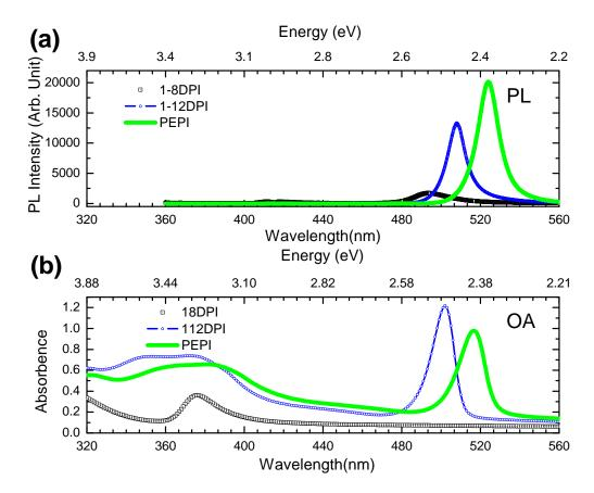
FIGURE 3.9: (a) OA and (b) PL of 18DPI, 112DPI lead iodide diammoniums based 2D layered perovskites. PEPI OA and PL spectra are reported as reference. The samples are excited with the 325 nm line of a HeCd laser at 1 mw in air.
