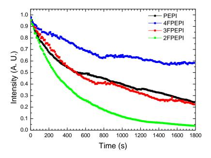
FIGURE 4.12: Photobleaching of iodide based perovskites layers deposited from 10wt% solutions. The measurement is carried on in air at room temperature, the laser power is 7 mW at 325 nm.
