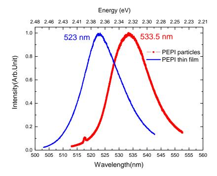
FIGURE 2.36: PL spectra of a 50 nm PEPI thin film (blue curve) and PEPI particles dispersed on quartz substrates (red curve). The excitation source is the 325 nm line of a HeCd laser.
