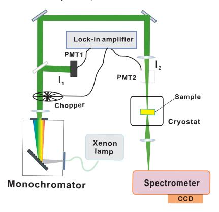
FIGURE 2.10: Experimental set-up of PLE measurement.
