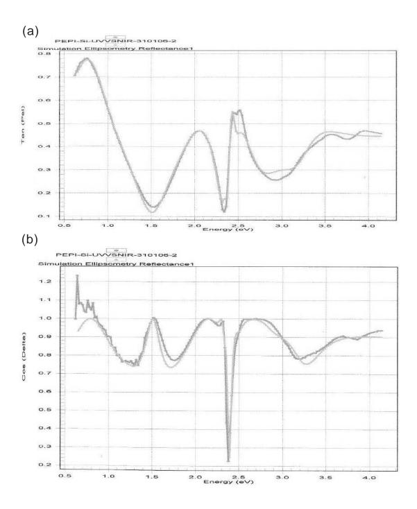
FIGURE 2.13: (a)  ${\rm Tan}\psi$  value and (b)  ${\rm Cos}\Delta$  value as a function of energy for a 240 nm PEPI thin film deposited on silicon substrate. Dark line is the experimental curve and the light line is the fitting curve given by software WINELLI II
