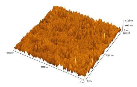
FIGURE 2.2: Topography of a PEPI thin film measured by AFM. Thickness of the film is estimated to be about 30 nm.
