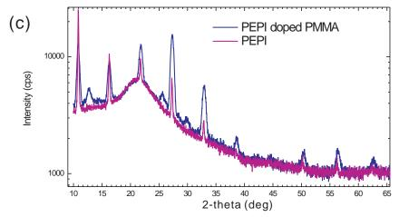
FIGURE 4.27: XRD spectrum of (a) a 641 nm PEPI doped PMMA layer and (b) a 1.1  $\mu m$  4FPEPI doped PMMA layer. (c) Comparison between XRD spectra of a 641 nm PEPI doped PMMA layer and a 50 nm PEPI spin-coated layer.
