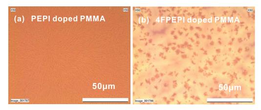
FIGURE 4.25: Optical microscope images of (a) a 641 nm PEPI doped PMMA layer and (b) a 1.1  $\mu$ m 4FPEPI doped PMMA layer.
