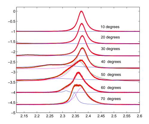
FIGURE 5.19: Angle resolved PL spectra of the PEPI standard cavity of Figure 5.18. The excitation source is the 325 nm line of a HeCd laser at 0.5 mW. PL intensities are normalized to 1, each PL curve is fitted by two lorentzian peaks (in magenta and blue); and the green curve is the sum of the two lorentzian peaks.
