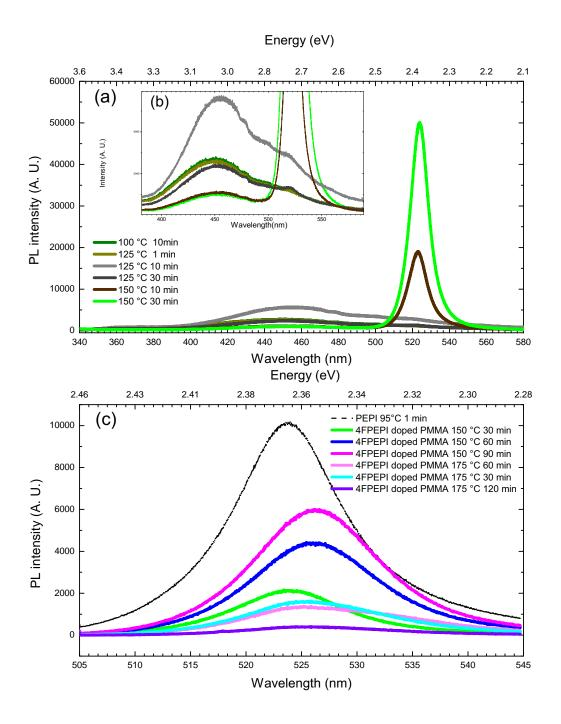
FIGURE 4.29: Comparative photoluminescence of (a) 4FPEPI doped PMMA annealed at 100 °C 10 min to 150 °C 30 min, the included graph (b) is a zoom of (a). (c) Comparative photoluminescence of 4FPEPI doped PMMA annealed at 150 °C 30 min to 175 °C 120 min. The PL spectrum of a PEPI thin film layer is drawn in the same graph for comparison. The excitation source is a 325 nm HeCd laser, the power is 10 mW. Measurement is carried at room temperature.
