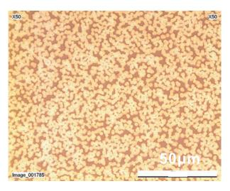
FIGURE 3.22: Microscope image of a 85 nm 4FPEB-PbI<sub>2</sub> thin film deposited by spin-coating on a quartz substrate.
