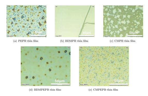
FIGURE 3.24: Images under microscope for PEPB, BDMPB and CMPB pure perovskites films and films obtained with their mixtures. Samples in (a), (b) and (c) are prepared from 1:10 solution of pure perovskite PEPB, BDMPB and CMPB respectively. (d) and (e) are mixed crystals of CMPEPB and BDMPEPB which are prepared by mixing two kinds of 1:10 solution of pure perovskites by 1:1 in volume
