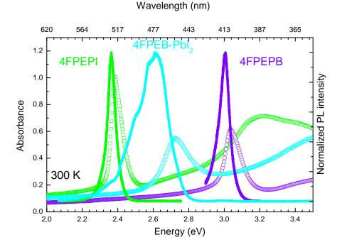
FIGURE 3.20: OA (scattered lines), PL (solid lines) spectra of 4FPEB-PbI<sub>2</sub>, 4FPEPI and 4FPEPB thin films. Experiments are carried on at room temperature. The PL intensities are normalized to 1, and the 325 nm line of HeCd laser is used as an excitation source for PL spectra.
