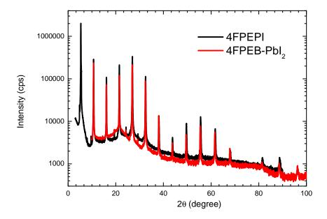
FIGURE 3.21: X-ray diffraction of a 4FPEB-PbI<sub>2</sub> (red line) and a 4FPEPI thin film (black line). The two samples, having a thickness of 85 nm and 50 nm respectively, are prepared by spin-coating.
