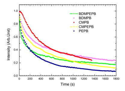
FIGURE 3.28: Evolution of PL intensity as a function of illumination time for PEPB, MFMPB, CMPB and their mixed perovskites CMPEPB and BDMPEPB thin films. The PL spectra are excited with a 325 nm line HeCd Laser at 5 mw in air.
