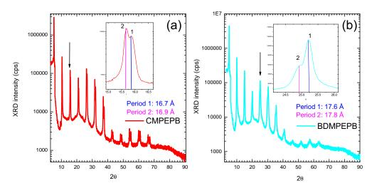
FIGURE 3.27: X-ray diffraction spectra of (a) CMPEPB and (b) BDMPEPB mixed perovskites thin films. The insert graphs are zooms of a particular single diffraction peak indicated by an arrow.
