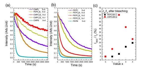
FIGURE 3.19: Photobleaching measurements at room temperature for (a) CMPC $_x$ B $_{4-x}$  and (b) for PEPC $_x$ B $_{4-x}$ . The laser power is kept at 7 mW, the excitation wavelength is 325 nm. (c) I $_{3600}$ /I $_0$  (as defined in the text), as a function of x.
