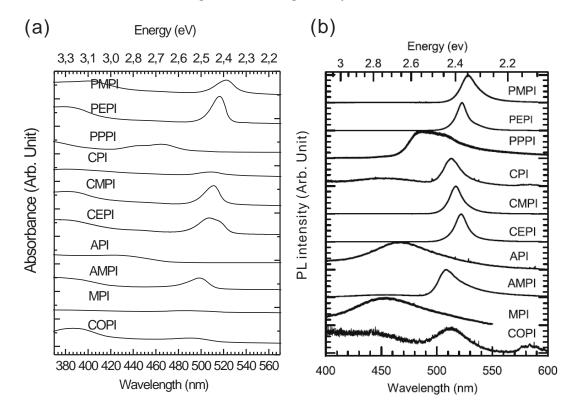
FIGURE 3.1: (a) Optical absorbance (OA) and (b) PL spectra of lead iodide 2D layered perovskites containing 10 different organic groups. PL curves are normalized. The curves are displaced vertically for clarity. The experiments are carried on at room temperature and the excitation source for PL is the 325 nm line of a HeCd laser, the power is 1 mW.
