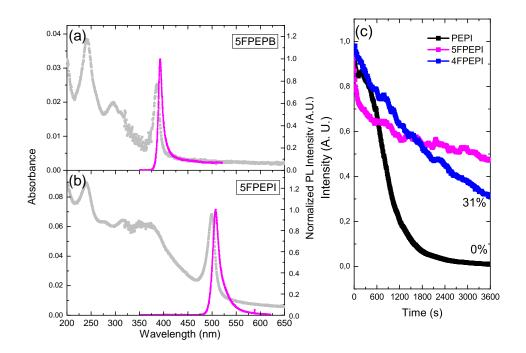
FIGURE 4.24: Comparative (a) absorbance, (b) normalized photoluminescence and (c) photobleaching rate of perfluorophenyl perovskite layers made from 10wt% solutions. The excitation laser is the 325 nm line HeCd laser. For the PL, the excitation laser power is 3 mW for 5FPEPB and 1 mW for PEPI. For the bleaching rate, the excitation laser power is 7 mW.
