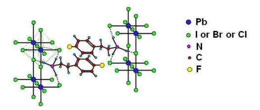
FIGURE 4.16: Sketch of the 3D structure of the  $(4-FC_6H_4(CH_2)_2NH_3)_2PbX_4$  (X = I or Br or Cl) perovskites.
