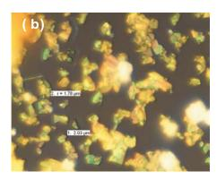
FIGURE 2.35: (a) PEPI particles dispersed in toluene solvent. Green luminescence is observed under UV lamp. (b) Photo under microscope for one drop of PEPI particles deposited on quartz substrate. The diameter of these crystals is around  $2\mu m$ .
