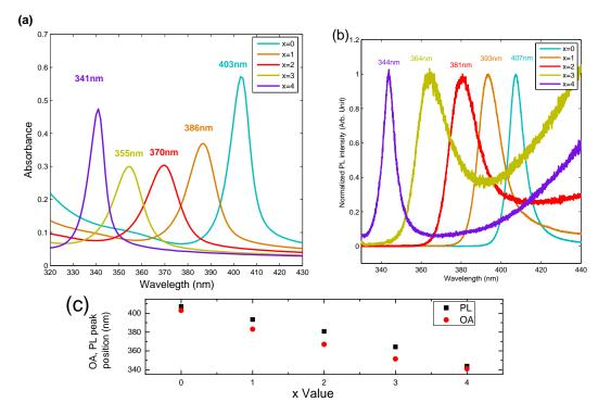
FIGURE 3.13: (a) Optical absorbance (OA) spectra and (b) Photoluminescence (PL) spectra of  $PEPC_xB_{4-x}$  thin films. PL spectra are normalized. The excitation source is the 325 nm line of a HeCd laser and the spectra are measured at room temperature. (c) Evolution of the resonance peaks positions as a function of x value.
