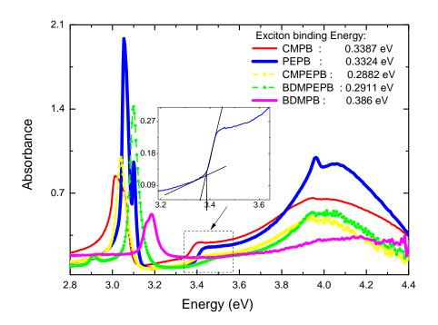
FIGURE 3.30: Absorption spectra for PEPB, CMPB, BDMPB, as well as CMPEPB and BDMPEPB at 10K in He environement. The insert graph shows the step-like structure around 3.4 eV for PEPB.
