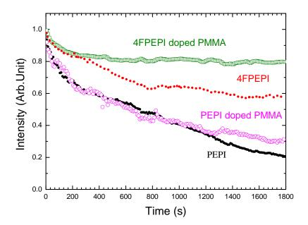
FIGURE 4.32: Photobleaching of 4FPEPI doped PMMA, 4FPEPI, PEPI doped PMMA, PEPI thin layers under the 325 nm line of a HeCd laser during 1800 s, the excitation power is 7 mW. The measurement is carried on at room temperature. The thickness of PEPI and 4FPEPI films are about 50 nm, PEPI doped PMMA and 4FPEPI doped PMMA layers are around 1  $\mu$ m.
