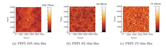
FIGURE 2.21: AFM images for PEPI thin films prepared from 10%, 4% and 1% solutions, and deposited on quartz substrate.
