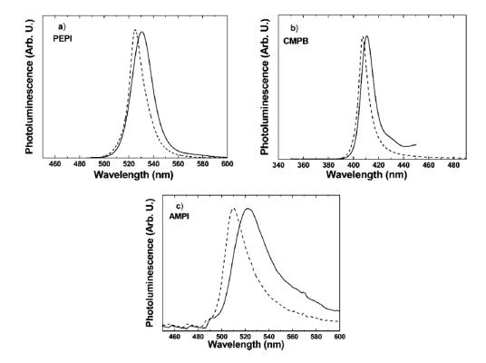
FIGURE 2.34: PL spectra of the three nanoparticles samples (solid lines) and of the spin-coated layers (dashed lines) obtained with the three perovskites (a) PEPI, (b) CMPB, and (c) AMPI. The excitation wavelength is 325 nm for AMPI and CMPB based samples and 405 nm for PEPI based samples. The PL curves have been normalized with their respective maximum intensities.
