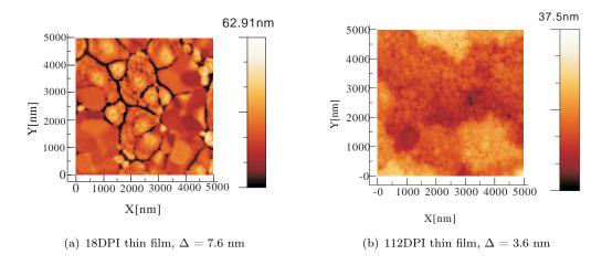
FIGURE 3.10: Topography of a 55 nm 18DPI thin film and a 51 nm 112DPI thin film.
