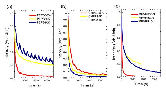
FIGURE 4.10: Evaluation of PL intensity as a function of time for thin films (a) PEPB (b) CMPB (c) MFMPB. The laser power is 10 mW at 325 nm, all samples are kept in He environment.
