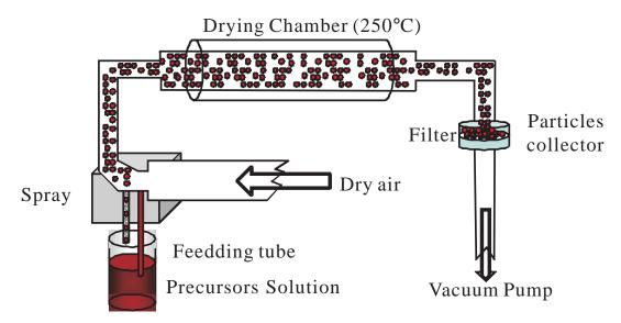
Figure 2.30: Sketch for the preparation of organic-inorganic perovskite nanoparticles by spray-drying method.
