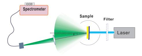
FIGURE 5.12: Schema of angle resolved photoluminescence experimental set-up.
