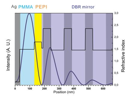
Figure 5.15: Profile of the electric field for the cavity mode energy 2.4 eV (blue line). The black curve presents the refractive index of the layers.
