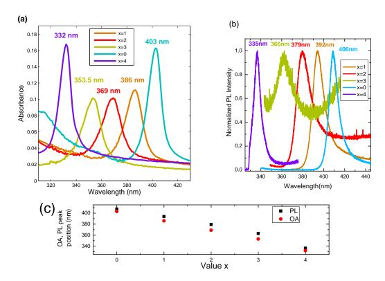
FIGURE 3.14: (a) Optical absorbance (OA) and (b) Photoluminescence (PL) spectra of  $\mathrm{CMPC}_x\mathrm{B}_{4-x}$ . PL spectra are normalized. The excitation source is the 325 nm line of a HeCd laser and the spectra are measured at room temperature. (c) Evolution of the resonance peaks positions as a function of x value.
