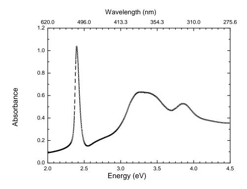
FIGURE 2.14: OA spectrum of a 50 nm thick PEPI film measured at room temperature.
