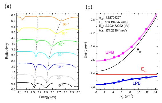
FIGURE 5.17: (a) Reflectivity and (b) dispersion curve of a PEPI cavity with anticrossing around  $k_{//} = 0 \ \mu m^{-1}$  (detuning  $\delta_{p-ex} = 0 \ \text{meV}$ ). The dashed line across dips in (a) are guides of eyes and the reflectivity curves are displaced along y axis for clarity
