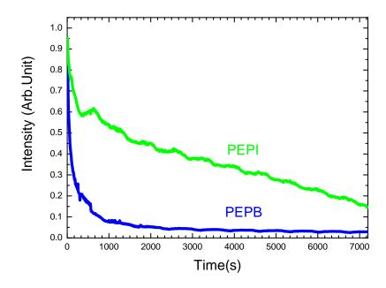
FIGURE 4.3: PEPI, PEPB thin films, thickness of several 10 nm, exposed under the 325 nm line of a HeCd laser at 10 mW. The measurement is carried on at 300 K in He environment.
