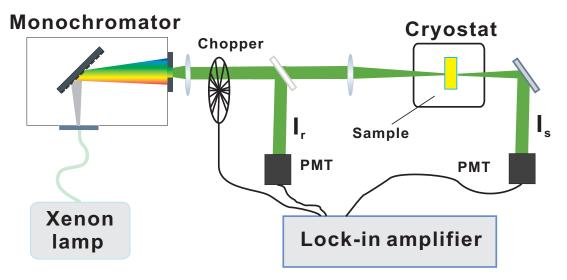
Figure 2.3: Experimental setup for optical absorbance measurement at low temperature.
