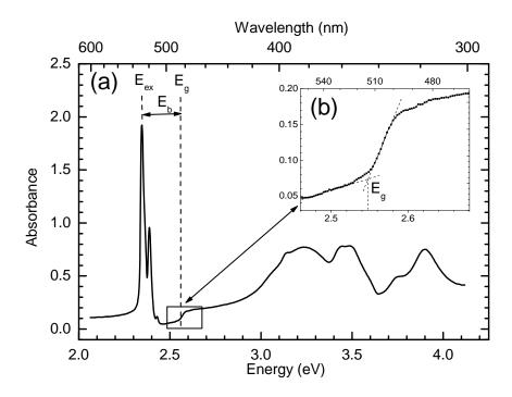
FIGURE 2.23: (a) OA spectra of 50 nm thick PEPI film measured at 10 K. The PL intensities are normalized. The inset (b) is a zoom of the square zone in order to see the energy gap. ( $E_{ex}$ ,  $E_g$ , and  $E_b$  represent the exciton energy, the energy gap, and the exciton binding energy, respectively.
