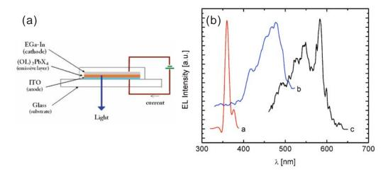
FIGURE 1.11: (a) Schematic representation of the LED device structure. (b) Electroluminescence spectra of the diodes  $ITO/(OL)_2PbX_4/$  Ga-In where X=Cl, curve a; Br, curve b; and I, curve c. Koutselas et al. (2011)
