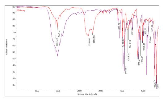
Figure 4.4: Infrared spectrum of PEI (magenta line) and heavy PEI (red line) ammonium salts.
