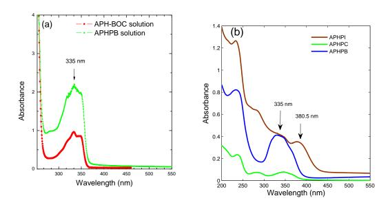
Figure 5.36: Absorbtion spectra of (a) two solution samples: APH-BOC and APHPB in DMF samples. (b) APHPX (X = Cl, Br and I) thin films
