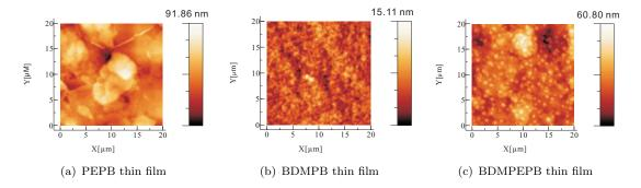
FIGURE 3.25: AFM images measured by taping mode for (a) PEPB, (b)BDMPB and (c) BDMPEPB thin films.
