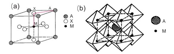
FIGURE 1.1: (a) Basic AMX<sub>3</sub> perovskite structure. (b) Sketch of a perovskite unit cell seen in three dimension(3D).
