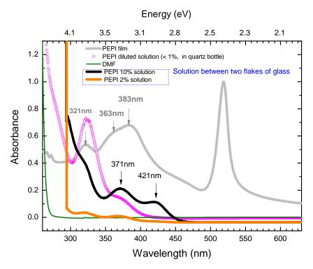
FIGURE 2.18: Absorbance of PEPI perovskites molecules dissolved in DMF solution. Measurement is carried on at room temperature. The grey line is the OA spectrum of a 50 nm PEPI thin film.
