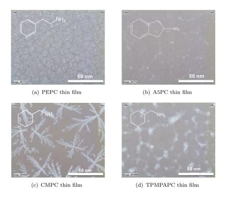
FIGURE 3.6: Images under microscope of PEPC, A5PC, CMPC and TPMPAPC thin films. The small chemical structures included in each image represent the corresponding organic amines in perovskites
