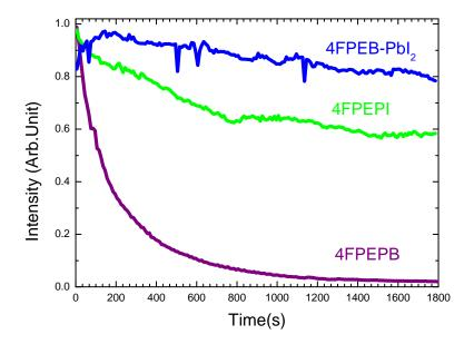
FIGURE 3.23: Comparison of photostability of 4FPEB-PbI $_2$ , 4FPEPB and 4FPEPI thin films. These three samples are prepared by spin-coating from their 10 wt% in DMF solution. The exitation source is the 325 nm line of a HeCd laser, the power is 7 mW.
