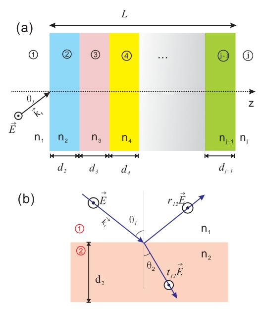
Figure 5.6: (a) Schema of a multi-layered structure. (b) A plan wave propagates from medium 1 to medium 2.
