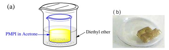
FIGURE 2.29: (a) Setup of slow solution exchange method and (b) a PMPI crystal grown by this method.
