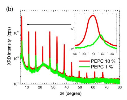
FIGURE 4.11: (a) Evaluation of PL intensity as a function of illumination time for two PEPC thin films prepared from 1% and 10% in DMF solution. The laser power is 7 mw at 325 nm. (b) XRD spectra of PEPC thin films prepared from 1% (green line) and 10% (red line) in DMF solution.
