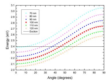
FIGURE 5.14: Simulation of the fundamental photon mode in a PEPI microcavity. PEPI layer is fixed to be 50 nm and the silver mirror is 30 nm. The curves in different colors correspond to different thicknesses of PMMA layer.
