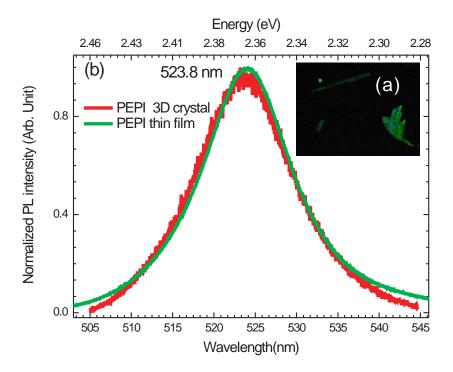
FIGURE 2.28: PL of PEPI crystal bulk grown from nitromethane/acetone mixted solution: (a) photo of the 3D crystals under a 312 nm UV lamp; (b) PL spectra measured at room temperature of the PEPI crystal bulk and of a 50 nm PEPI thin film. The PL intensity is normalized, the excitation laser is HeCd at 325 nm, with incident power of 0.6 mW. The normalized PL of a PEPI thin film is drawn for comparison.
