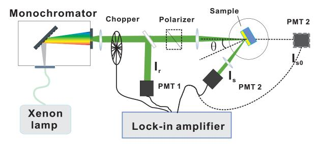
FIGURE 5.11: Schema of the angle resolved reflectivity experimental set-up.
