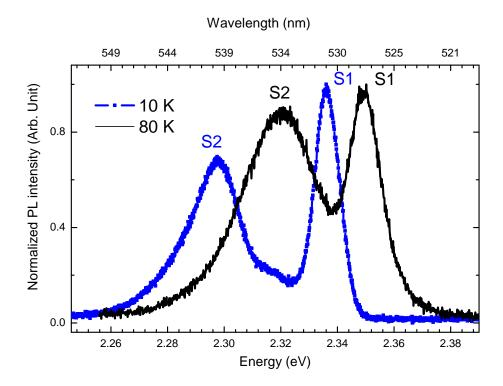
FIGURE 2.24: PL spectra of a 50 nm PEPI thin film at 10 K and 80 K. The PL intensities are normalized. The sample is placed in He bath in cryostat, the excitation source is Xenon lamp at 467 nm
