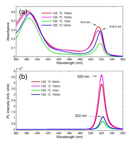
FIGURE 4.31: Comparative (a) absorbance, (b) photoluminescence of PEPI doped PMMA layers made from 20wt% solutions. For the PL, the excitation source is the 325 nm HeCd laser, the power is 10 mW. Measurement is carried at room temperature.
