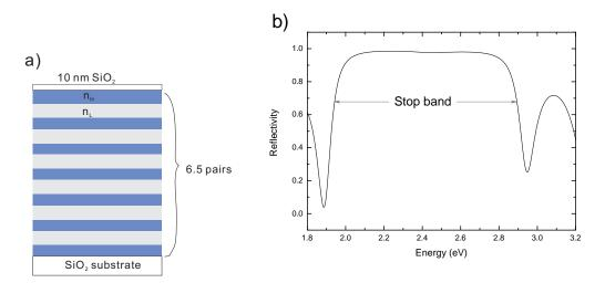
FIGURE 5.3: a) Structure of a DBR fabricated by Layertec. The blue bands represent the layers with  $n_H = 2.36$  and the light grey bands represent the layers with  $n_L = 1.46$ ; b) simulated reflectivity of a DBR fabricated by Layertec. The stop band is centered at 515 nm at normal incidence.
