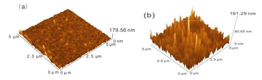
FIGURE 4.18: AFM pictures of (a) the 2FPEPI layer, (b) the PEPI layer, obtained by tapping mode. Be careful that the vertical scales are different in these two images.
