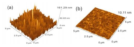
FIGURE 5.22: AFM images of (a) a 50 nm PEPI layer and (b) a 350 nm 4FPEPI doped PMMA layer.
