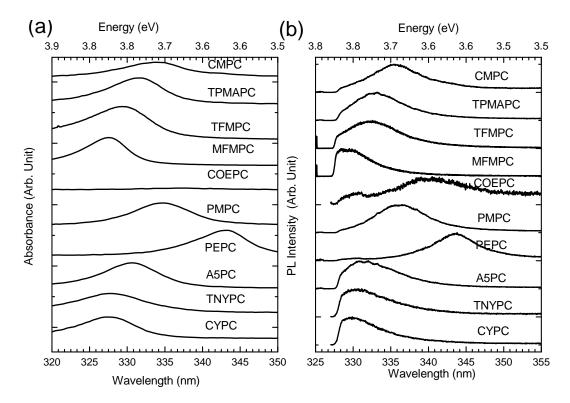
FIGURE 3.3: (a) Optical absorbance (OA) and (b) PL spectra of lead chloride 2D layered perovskites containing 10 different organic groups. PL curves are normalized. The curves are displaced vertically for clarity. The experiments are carried on at room temperature and the excitation source for PL is the 325 nm line of a HeCd laser, the power is 1 mW.
