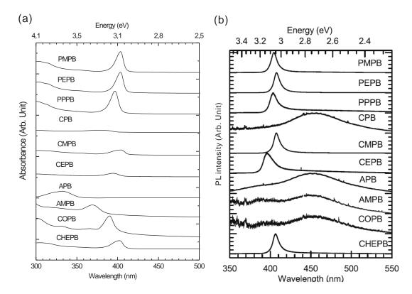
FIGURE 3.2: (a) Optical absorbance (OA) and (b) PL spectra of lead bromide 2D layered perovskites containing 9 different organic groups. PL curves are normalized with their respective maximum intensities. The curves are displaced vertically for clarity. The experiments are carried on at room temperature and the excitation source for PL is the 325 nm line of a HeCd laser, the power is 1 mW.
