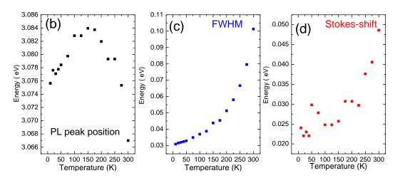
FIGURE 3.31: (a) OA (blue line) and PL (red line) spectra of BDMPEPB from 10 K to 300 K. (b) PL peak position (c) FWHM (d) Stokes-shift as a function of temperature. The excitation source for PL is the 325 nm line of HeCd laser, the power is 0.2 mW.
