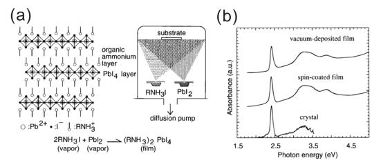
FIGURE 1.8: (a) Schematic representation of the structure of layered perovskites  $(RNH_3)_2PbI_4$  and preparation process of layered perovskites using the dual-source vapor deposition. (b) The absorption spectrum of the co-deposited film of  $PbI_2$  and phenethylammonium iodide. The absorption spectra of the spin-coated film and the crystal of the layered perovskite with phenethylammonium layer are also shown. Era et al. (1997)
