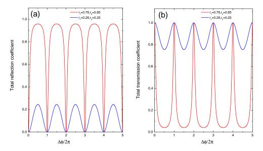
FIGURE 5.2: Total reflection (a) and transmission (b) coefficients for two sets of parameters:  $r_1$ =0.78,  $r_2$ =0.85 (in red);  $r'_1$ =0.28,  $r'_2$ =0.25 (in blue).
