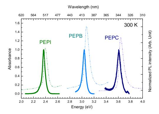
FIGURE 2.6: PL (solid lines) and OA (dashed lines) spectra of PEPI, PEPB and PEPC thin films at room temperature. The excitation is the resonant line 325 nm of a HeCd laser.
