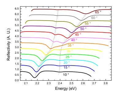
FIGURE 5.25: Reflectivity spectra of 4FPEPI doped PMMA cavity, for different angles of incidence. The dotted lines are guides to eyes. The quality factor is estimated to be about 36.
