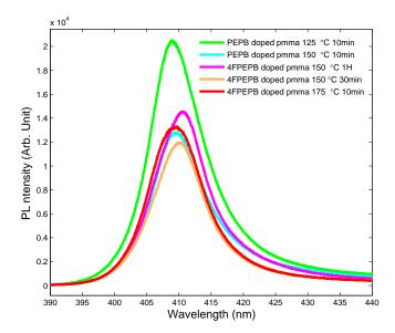
FIGURE 4.30: Comparative photoluminescence of PEPB doped PMMA layer and 4FPEPB doped PMMA annealed at different conditions. The excitation source is a 325 nm HeCd laser, the power is 10 mW. Measurement is carried at room temperature.
