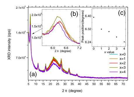
FIGURE 3.11: (a) X-ray Diffraction pattern for  $PEPC_xB_{4-x}$  mixed perovskites fabricated on quartz substrate. The solutions used for deposition are 0.05 mol/L. The insert graph (b) is the a zoom of the first peak around 6.35°. The insert graph(c) shows the evolution of the peak position of the first mode versus x value.
