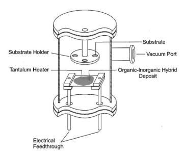
FIGURE 1.9: Schematic cross section of a single source thermal ablation chamber. Mitzi et al. (1999)
