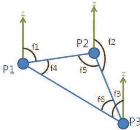
Figure 2.7: Diagram explaining the 3D invariant construction. The 3 points described ( $P_1$  to  $P_3$ ) and their triangle are in blue.  $f_1$  to  $f_6$  are the angles used as features. The 3 vertical green arrows represent the vertical axis.
