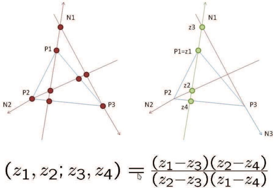
Figure 2.6: Left: diagram illustrating the features used in the proposed projective-invariant potential. In order to describe the blue triangle, we build three red lines with four points on each. Right: in order to describe one of these lines (the green one), we denote the four points by  $z_1$  to  $z_4$  (complex numbers). Bottom: we use the cross ratio formula to compute one descriptor for each of the three lines.
