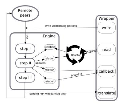
Figure 5.3: Wrapper running in parallel with Webdamlog stage
