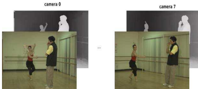
Figure 4.4: MVD representation, each view is composed of a texture image and a depth map.
