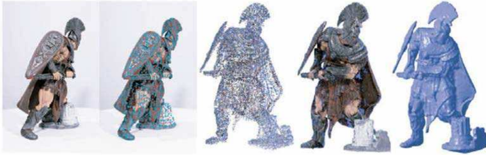
Figure 4.8: From left to right: A sample input image, detected features, reconstructed patches after the initial matching, final patches after expansion and filtering, and the mesh model [Furukawa and Ponce, 2010].
