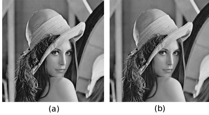
Figure 4.4: (a) Natural image and its estimation keeping only 10% of its wavelet coefficients (b).
