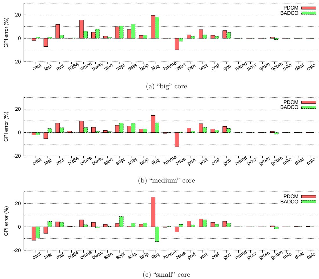
Figure 3.6: CPI error of PDCM and BADCO for the "small", "medium" and "big" cores, with the uncore configuration "001".
