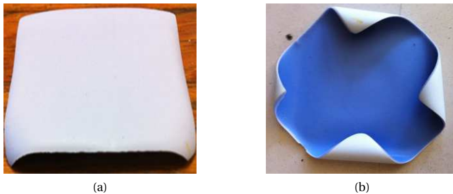
Figure 2.46: Integration of one ESL41060 layer in six ESL41110 layers: (a) With ESL41060 firing profile. (b) With ESL41110 firing profile
