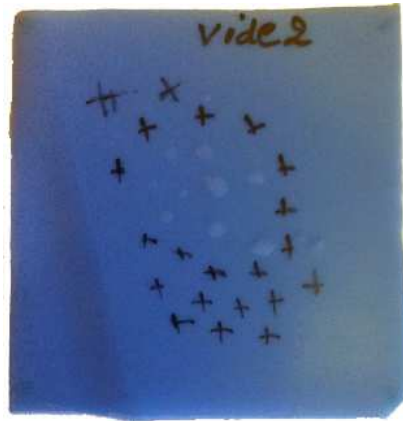
Figure 2.38: The LTCC circuit "vide 2" composed of six empty ESL41110 layers for preconditioning effect verification on the substrate shrinkage
