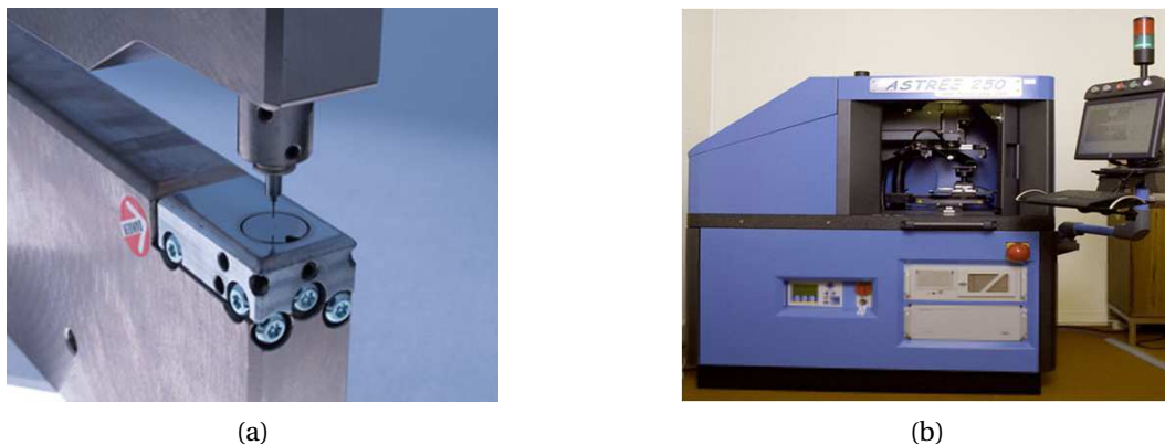
Figure 2.8: Via and cavity formation tools: (a) Mechanical puncher system (source IMST). (b) Our Nd-YAG laser system
