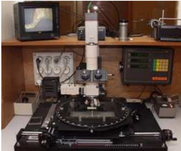
Figure 2.25: 3D optical measuring microscope used in our laboratory
