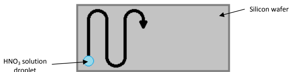
Fig A13. Schematic diagram of the collection of impurities on the surface of silicon wafer by a HNO 3 droplet
