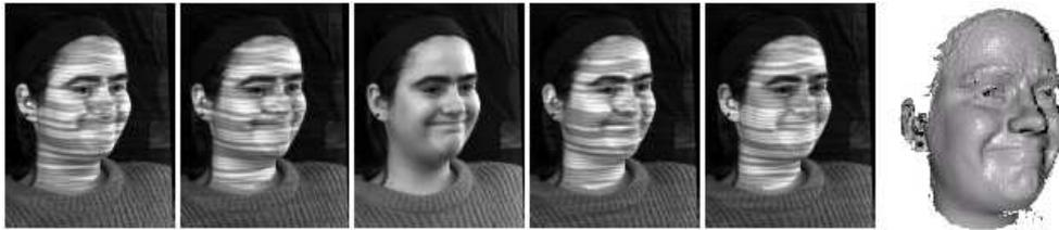
**Figure 3.3:** *An example of structured light reconstruction from [ZSCS04].*
