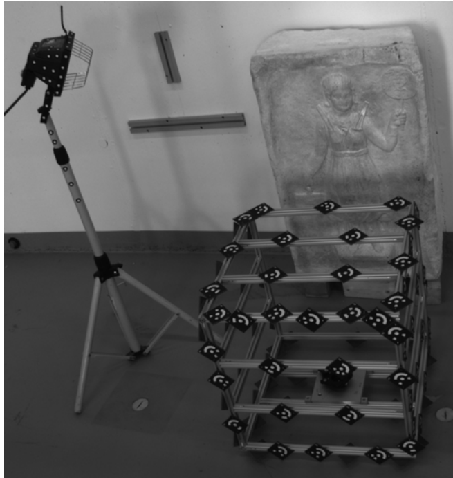
Figure 6.3: Acquisition of the position of the light sources.
