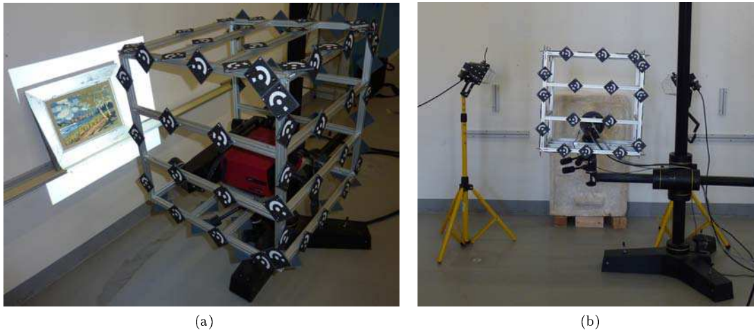
Figure 5.1: Multisensor acquisitions using the target frame. (a) Detail of the cross-stitch canvas 3D digitization. (b) Detail of the plaster bas-relief multispectral acquisition. Even though the ring-light is still fixed to the multispectral camera, only the two halogen lights are used during the acquisitions.
