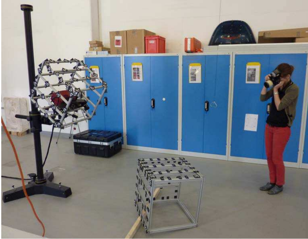
Figure 4.15: Calibration between the target frame and the Gom Atos III. The target-covered object used for the calibration is shown on the floor.
