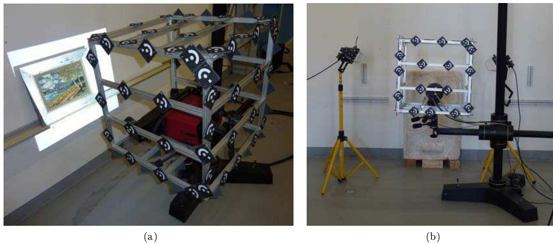
Figure 5.1: Multisensor acquisitions using the target frame. (a) Detail of the cross-stitch canvas 3D digitization. (b) Detail of the plaster bas-relief multispectral acquisition. Even though the ring-light is still fixed to the multispectral camera, only the two halogen lights are used during the acquisitions.
