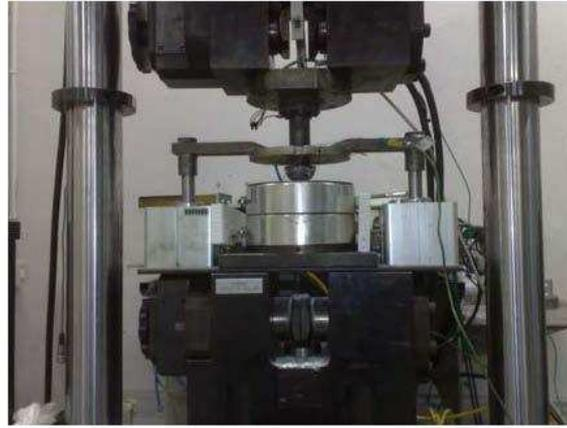
Figure 1.23: Warm Nakazima forming test [64]
