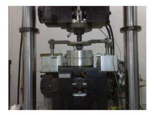
Figure 1.23: Warm Nakazima forming test [64]
