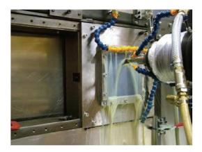
Figure 1.3: Single point incremental sheet forming setup
