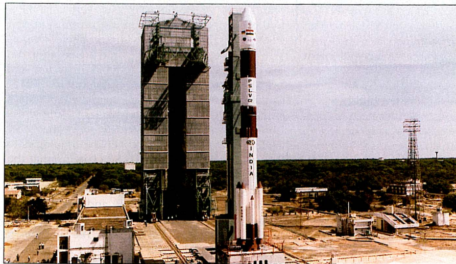
The PSLV sparked development of a ground segment and infrastructure, including a 3,000-tonne mobile service tower for vertical integration of the launcher and payload.
