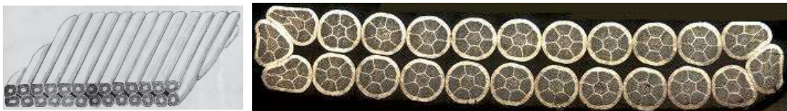
Figure 2.11: Schematic view of Rutherford cable [53] (left). Cross section of a Bi-2212 Rutherford cable [54] (right).
