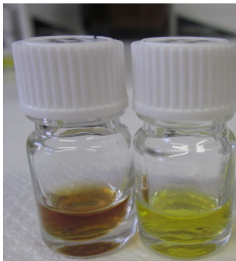
Figure 35. Optical photograph of 60 mM \text{H}_2\text{PtCl}_6 (right) before adding L-DOPA and (left) after adding L-DOPA.
