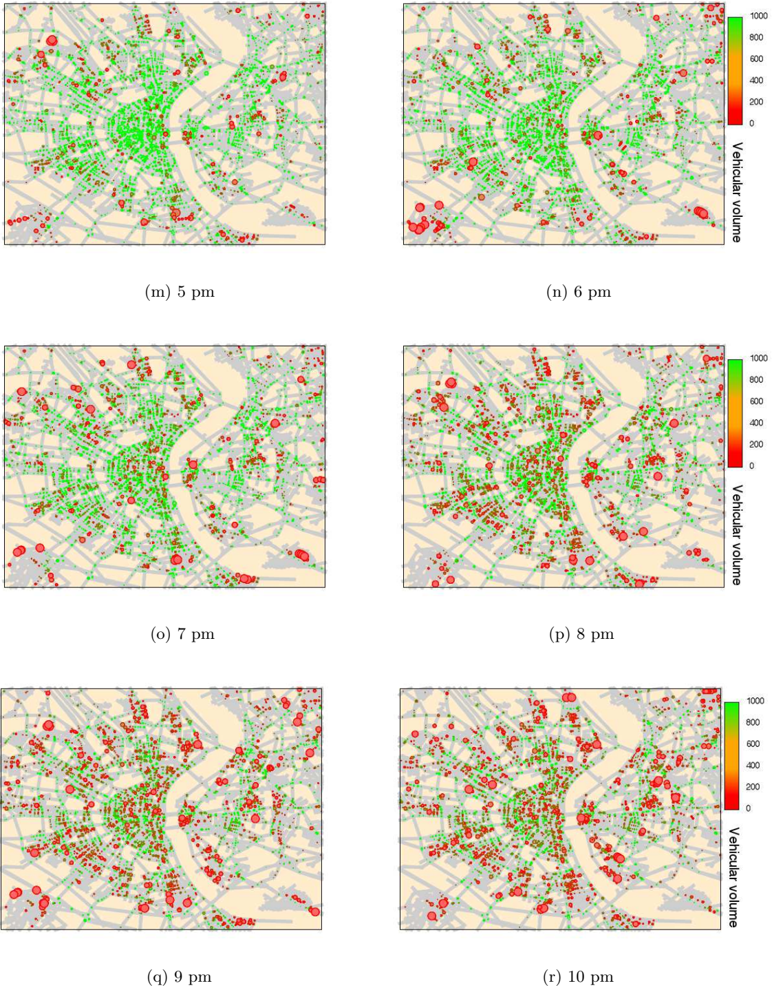
Figure 5.19: Road network: Spatiotemporal distribution of order-2 prediction error and vehicular volume (5 pm to 10 pm)
