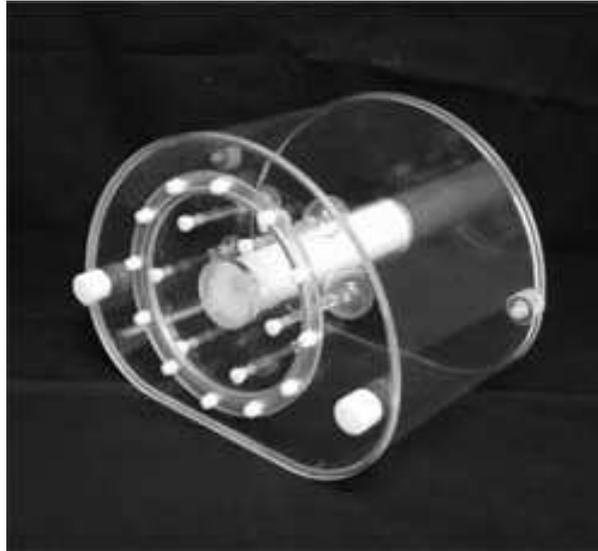
Figure 6.16 – Fantôme NEMA IEC (Data Spectrum Corporation, Hillsborough, NC, USA) contenant six sphères.
