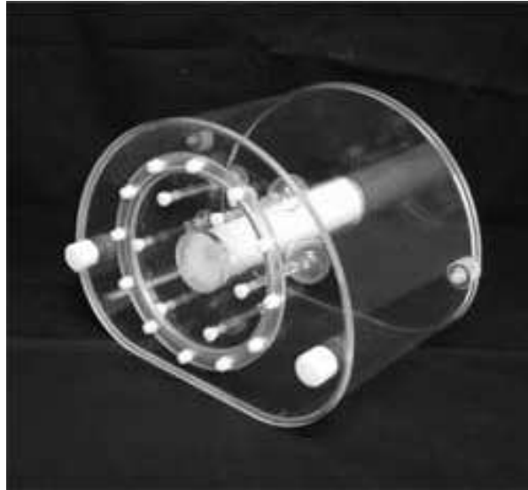
Figure 6.16 – Fantôme NEMA IEC (Data Spectrum Corporation, Hillsborough, NC, USA) contenant six sphères.
