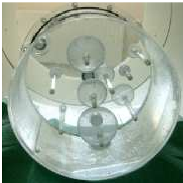
Figure 2.1 – Fantôme cylindrique de Jaszczak (Data Spectrum Corporation, Hillsborough, NC, USA) contenant 9 sphères.
