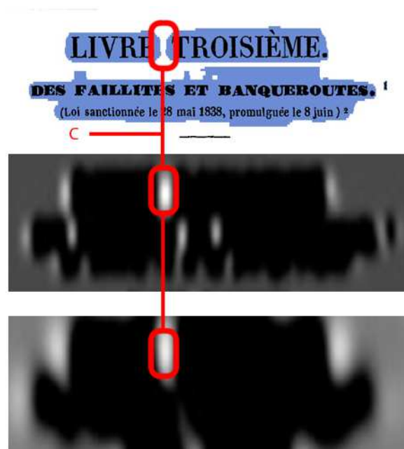
Figure 4.14: This figure displays a serious problem when the title of the page divides into two isolated text regions. Currently there is no fix for his problem and the use of morphological opening is not recommended to solve it.
