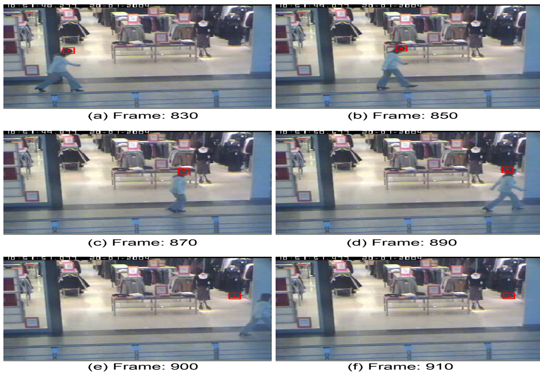
Figure 5.14: SIFT point tracking failure due to small size of the person's image, the proximity of the SIFT point to the person contour and to the low texture on the containing region. The SIFT point (red cross) is tracked correctly until frame 890, where it clings on the background which presents similar descriptor region (red square) at this location
