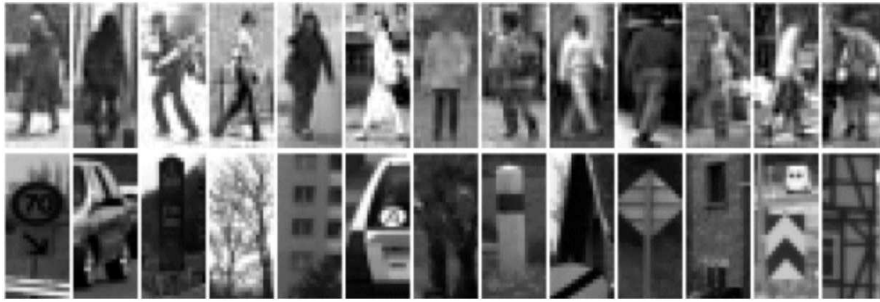
Figure 7.2: Samples from DaimlerChrysler dataset. The first row consists of some examples of annotated people. The second row consists of some cropped negative samples with the same size as annotated people ( 18 \times 36 pixels)
