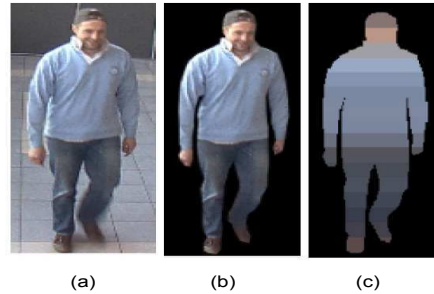
Figure 2.40: Color-position histogram [Truong Cong 2010]: (a) original image; (b) localization of the silhouette; (c) color distribution in the silhouette.
