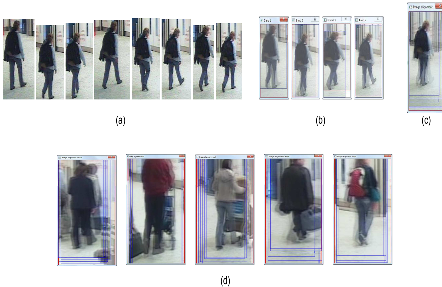
Figure 6.7: Image alignment process illustration and results on iLids-AA dataset samples. In the first row, the alignment process is detailed: (a) 8 sampled images of the same person obtained by automatic people detection and tracking. The person is not delimited and centred correctly in images (various shifting). (b) Samples of alignment of successive pairs of images. (c) The final alignment results. (d) Some other results of people images alignments. In this figures, red bounding box corresponds to the first image of each set of images (defining the origin of coordinate system), and the blue bounding boxes are those of the remaining images of each set. Image transparencies have been modified to show the alignment results.
