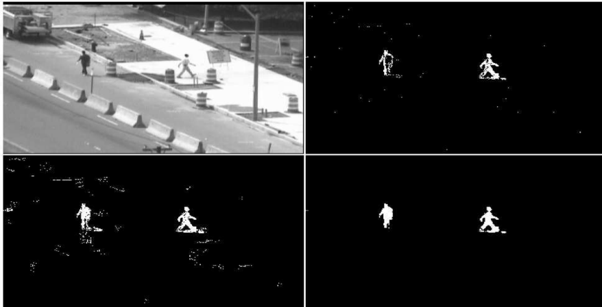
Figure 5.1: Background subtraction results for real video. The top-left image is the original one, the three other images are the results of background subtraction using different parameter values [McHugh 2009]
