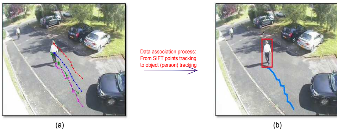
Figure 5.20: From SIFT point tracking to Object (Person) tracking: (a) four SIFT points at different location of the person body are tracked using particle filter. (b) The person tracking result after data association step.
