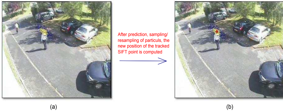
Figure 5.17: Tracking of one SIFT point on the head of a person by particle filter: (a) the predicted position of all particles in blue and yellow. The yellow particles are the sampled ones, which will be used to generate new ones to replace degenerated particles in blue. (b) in red, the new location of the tracked SIFT point, computed as the barycentre of all weighted sampled particles.
