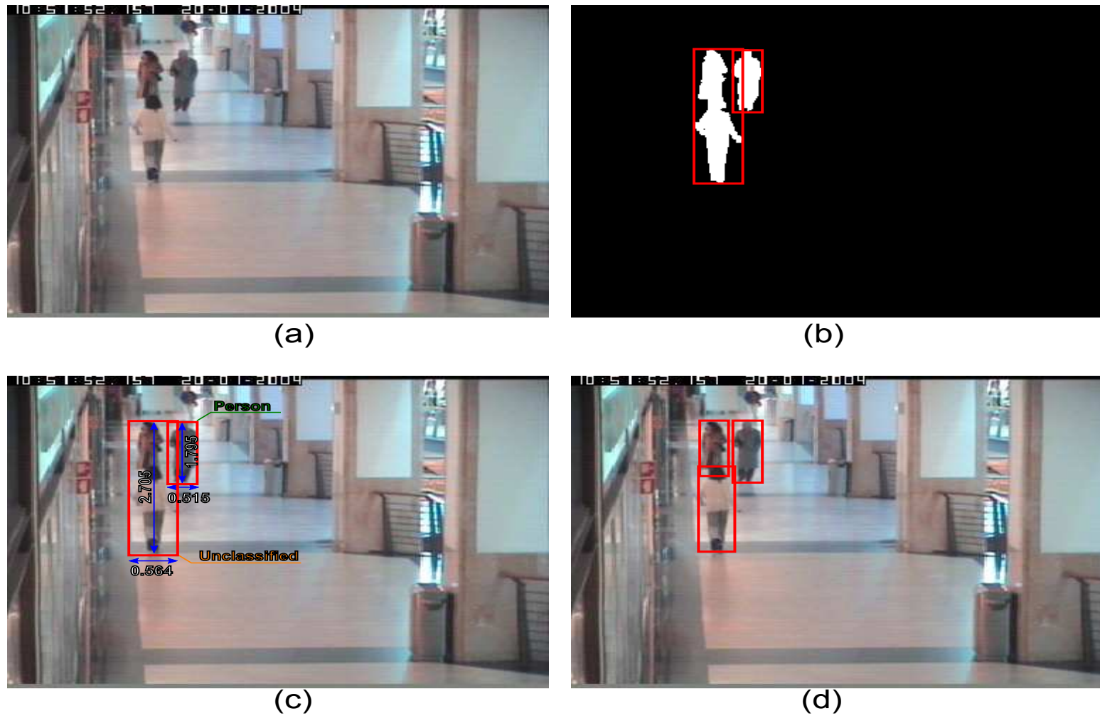
Figure 5.8: Use of people detector to split grouped persons. (a) Original frame. (b) Background subtraction result. Two persons are grouped due to the connected foreground pixels. (c) Failure of the classification of grouped people by real dimension estimation. (d) Result of our people detector applied in the restricted area of unclassified object (by real dimension estimation)
