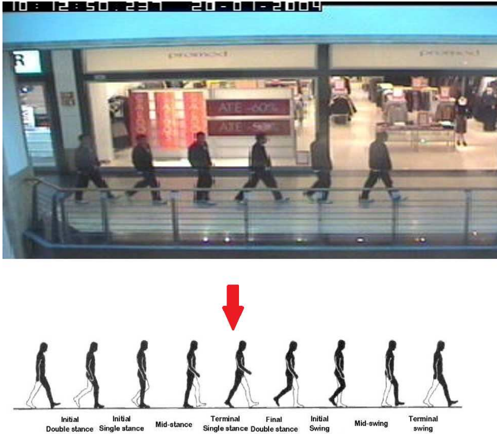
Figure 1.7: Gait recognition: gait is decomposed into different identifiable phases which are processed. No collaboration from people is required.
