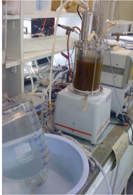
Figure 12 – The system of gas measurement (foreground) adapted to the bioreactor (background).
