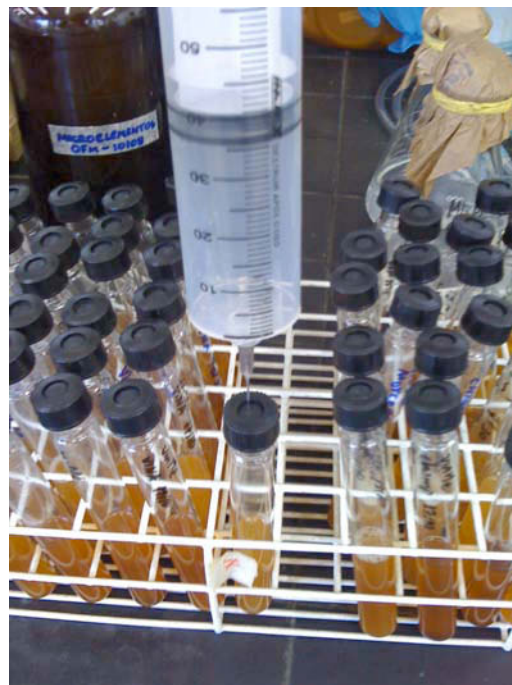
Figure 8 – The use of a graduated syringe in the quantification of the gas produced during fermentation
