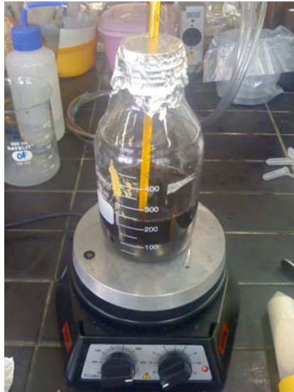
Figure 6 - Technique of producing an anaerobic medium. Boiling under anoxic environment is one important step.
