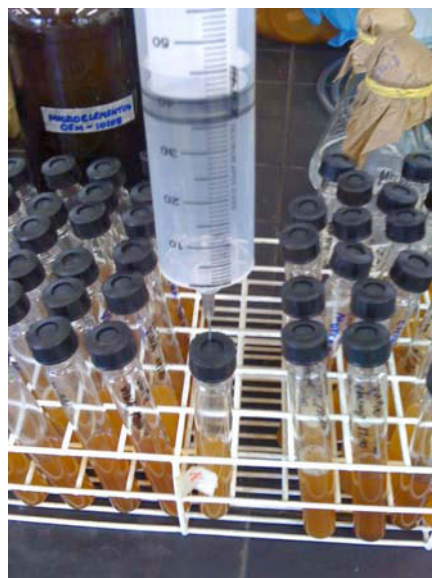
Figure 7 - Biogas quantification using a 60ml syringe.
