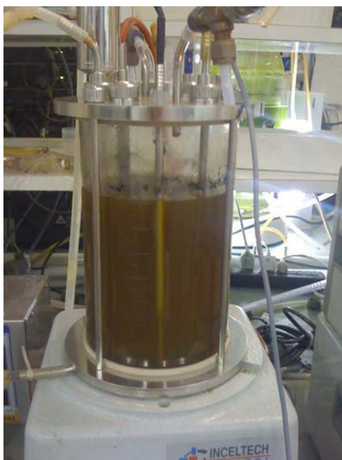
Figure 11 – 2L Bioreactor used in scaled up production of biohydrogen and VFAs by the consortium LPB AH2 (cultivated in vinasse medium supplemented with sugarcane molasses) and LPB AH1 (cultivated in vinasse medium supplemented with sugarcane juice).
