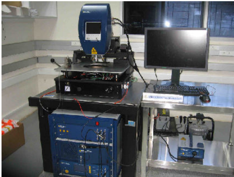
FIGURE 5.11 – MEMS Analyzer MSA-500 de la société Polytec.
