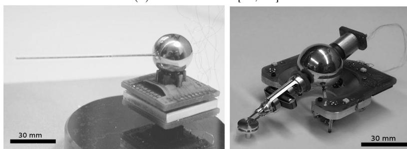
(b) Microrobot MINIMAN utilisant le stick-slip [88, 42].
