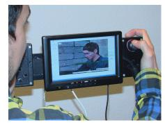
**Figure 4.16** – Our hand-held virtual camera device with custom-built dual handgrip rig and button controls, a 7-inch LCD touch-screen.
