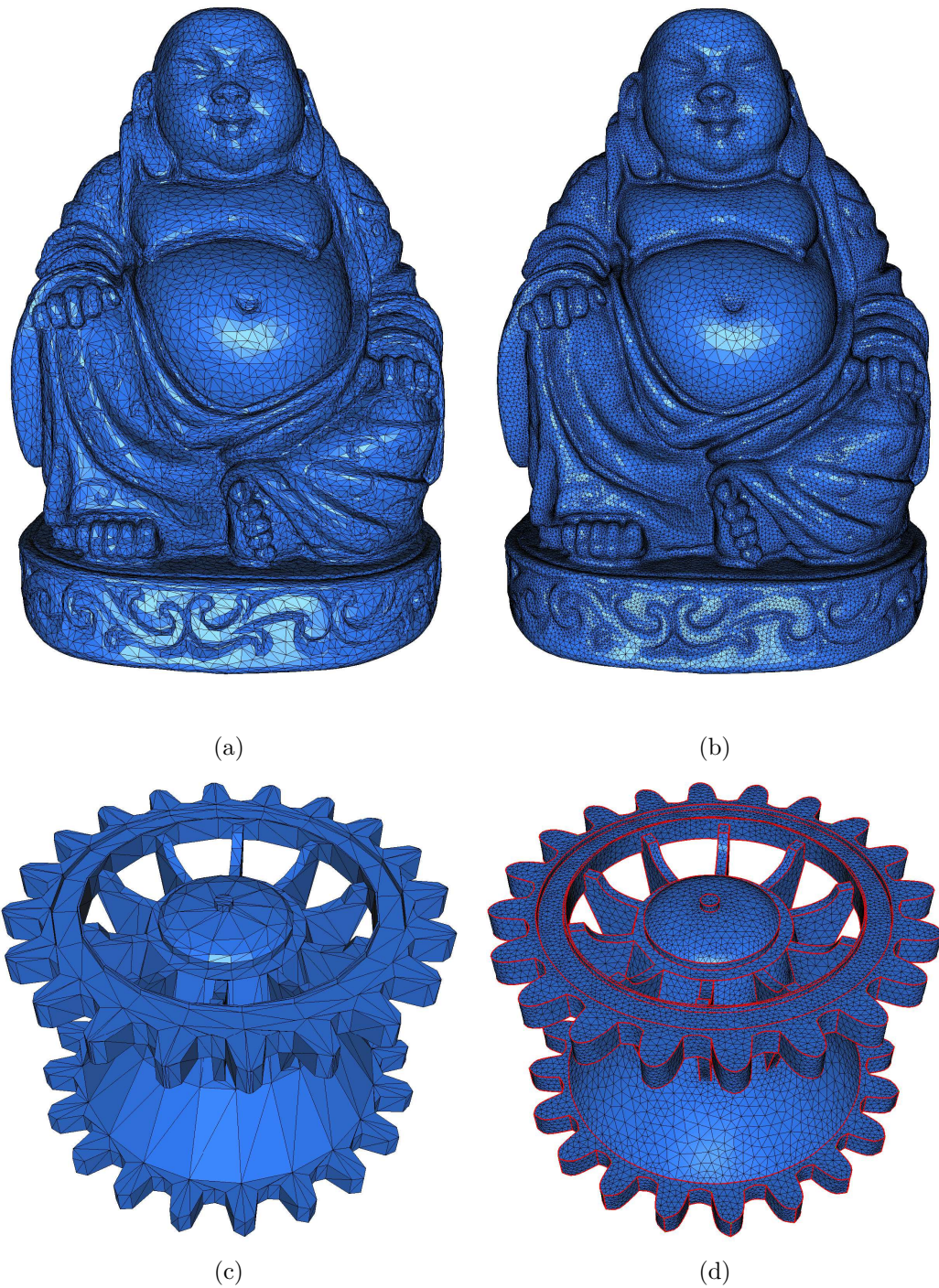
Figure 8.17: (a-b) Remeshing of the buddha model, enclosed in a bounding box of dimensions 99.3304 \times 141.9974 \times 93.2093 . Here we take h_{min} = 0.5 , h_{max} = 10 , h_{grad} = 1.2 , and \varepsilon = 0.2 ; (a) initial triangulation; (b) remeshed triangulation. (c-d) Remeshing of the drwL model, enclosed in a bounding box of dimensions 141.9963 \times 27.0421 \times 74.2486 , with h_{min} = 0.1 , h_{max} = 5 , h_{grad} = 1.2 , and \varepsilon = 0.05 ; (c) initial triangulation; (d) remeshed triangulation.
