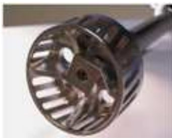
Figure 2. Picture of the mixed head of a typical rotor-stator system
