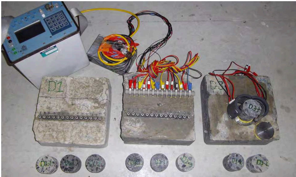
Figure 9.1: Testing of Mix D1, D2 and D3 with the resistivity cell (cores) and the surface resistivity probe (slabs).
