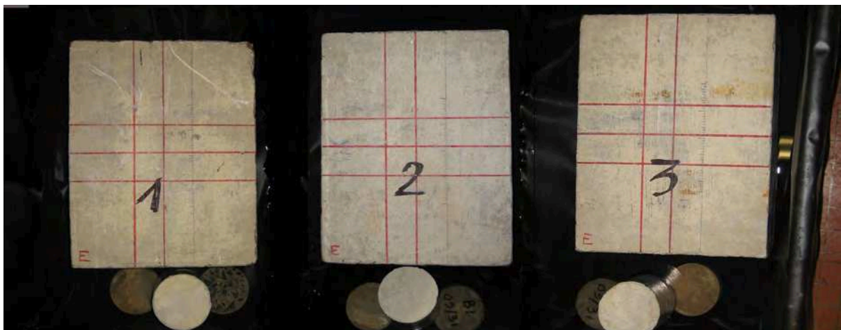
Figure 9.6: Conditioning of concrete slabs and witness cores (for gammadensimetry) for Slabs 1 (0 g/L NaCl), 2 (15 g/L NaCl) and 3 (30 g/L NaCl) , temp. 20°C and RH 80%.
