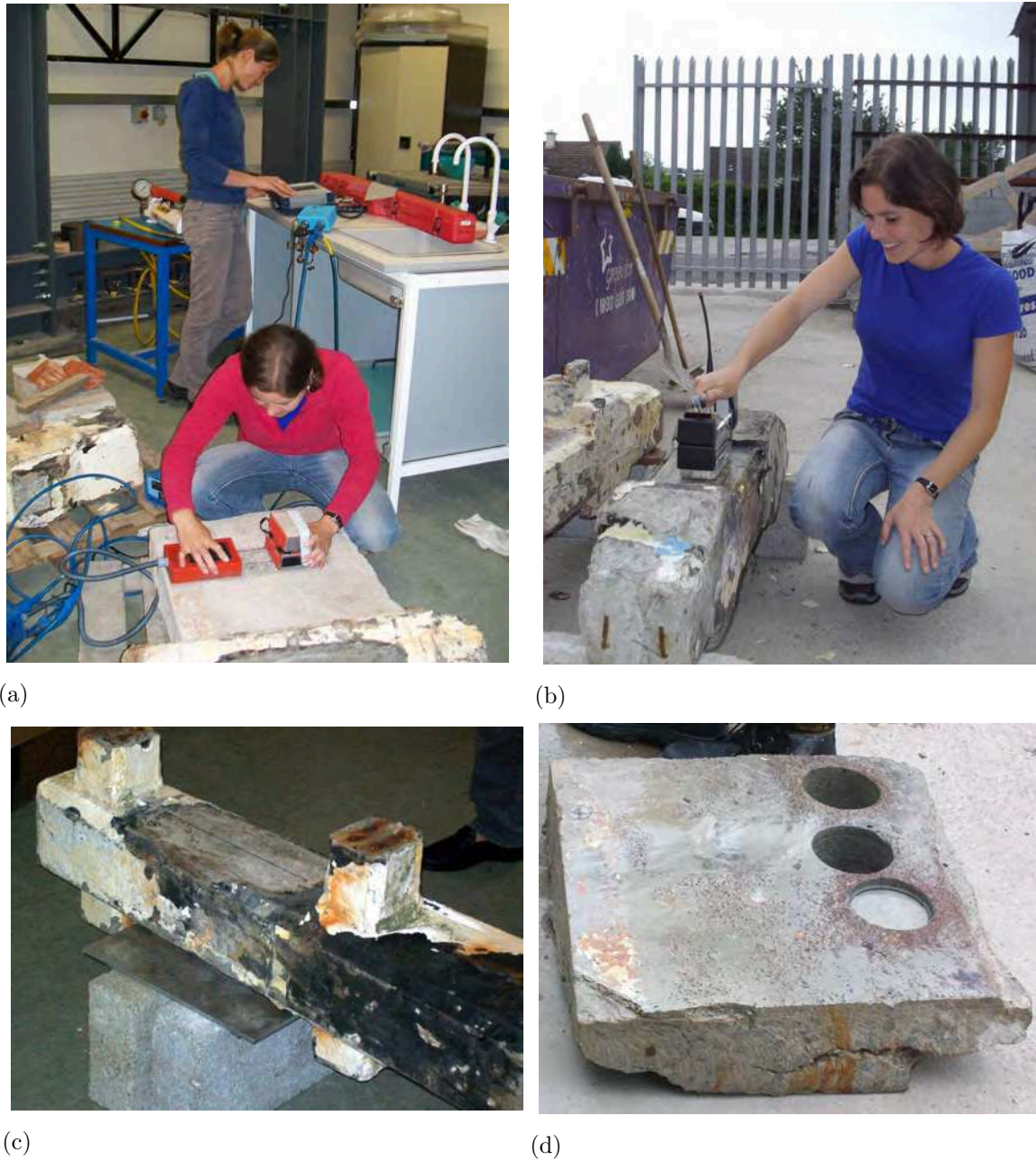
Figure 9.17: Testing of concrete elements from the dismantled Mizen Head footbridge with showing (a) WARR GPR measurements on a slab element, (b) capacitive probe measurements of a hanger, (c) a hanger where the protective paint and bituminous coating had been removed for resistivity testing and (d) a slab element from which core specimens had been taken for non-destructive testing (chloride diffusion coefficient).
