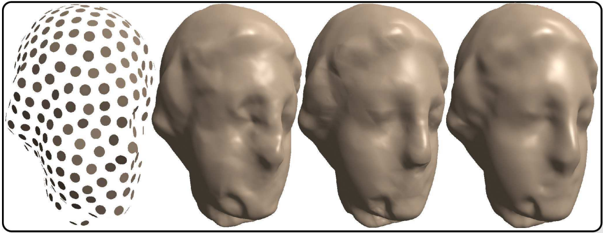
Figure 8: The Igea model uniformly sampled by 600 points is refined to 150k points with various techniques. From left to right: the butterfly (after a meshing step), the Guennebaud et al. diadic refinement and our new \sqrt{3} -like refinement.
