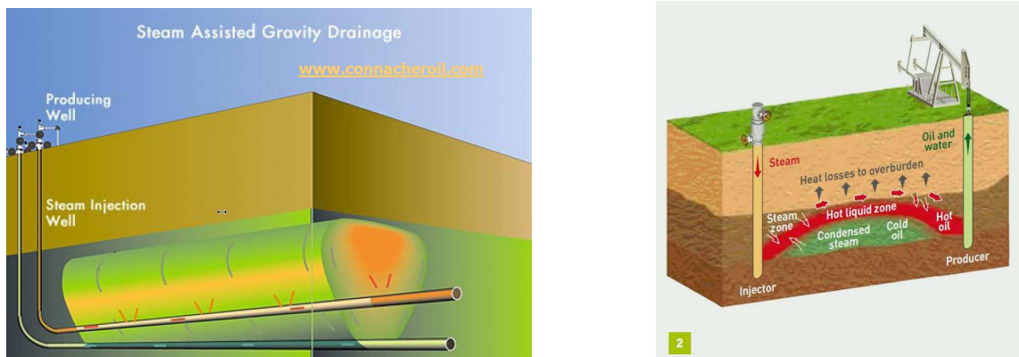
Figure 3 – Thermal methods for heavy oil production: SAGD (left) and Steam Drive (right) process.
