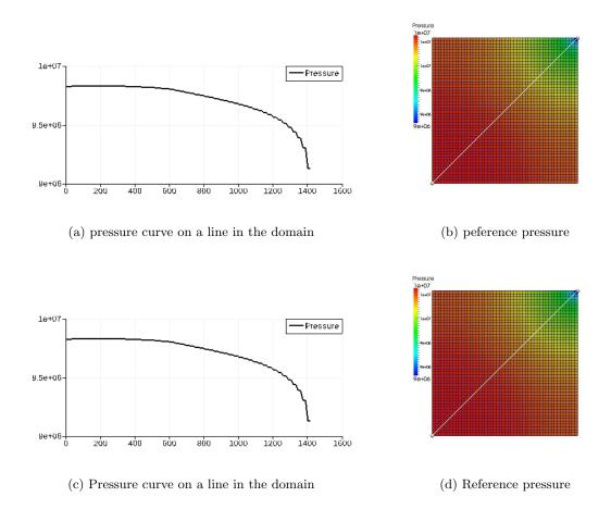
Figure 2.5: Reference pressure, classical (top) vs. adaptive (bottom) resolution at time 50 months for the test case of Section 2.5.2
