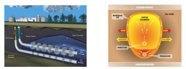
Figure 4.1: SAGD process: wells (left) and steam chamber (right).
