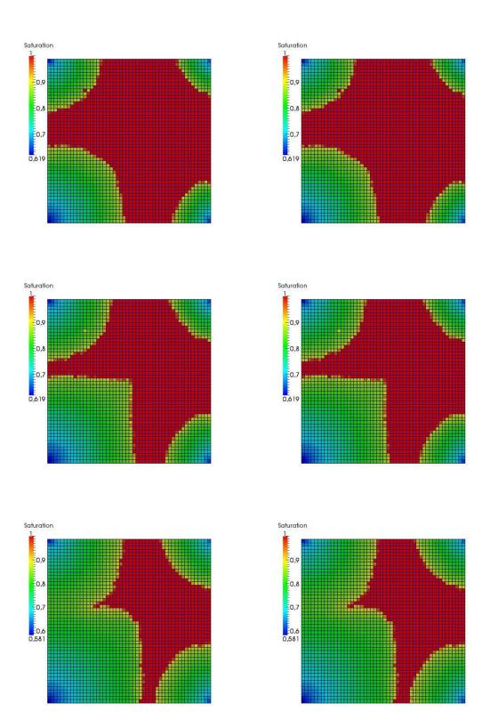
Figure 2.25: Liquid saturation, classical (left) and adaptive (right) resolutions at times 7 years, 10 years, and 15 years for the test case of Section 2.5.4.1
