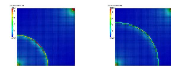
Figure 2.6: Spatial error distribution at times 30 months and 40 months for the test case of Section 2.5.2
