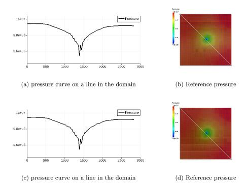
Figure 2.27: Reference pressure, classical (left) and adaptive (right) resolution at time  $5.2 \times 10^7$ s for the test case of Section 2.5.4.1
