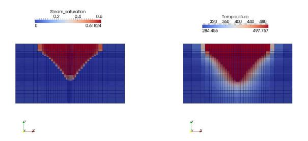
Figure 4.7: Expansion of the steam chamber: steam saturation (left) and temperature of the reservoir (right) at 2000 days.
