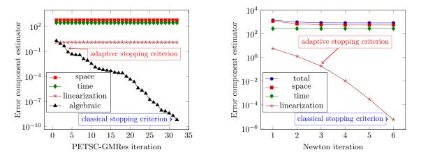
Figure 2.2: Evolution of the spatial, temporal, linearization, and algebraic error estimators (2.4.20) for all components for a fixed mesh at time  $1.04 \cdot 10^6$ s, as a function of GMRes iterations on the first Newton iteration (left) and of Newton iterations (right)
