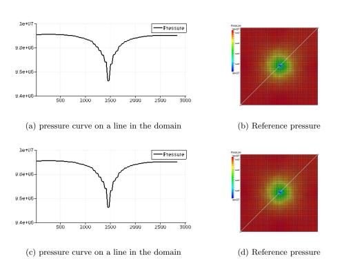
Figure 2.34: Reference pressure, classical (top) and adaptive (bottom) resolution at time 8 years for the test case of Section 2.5.4.2
