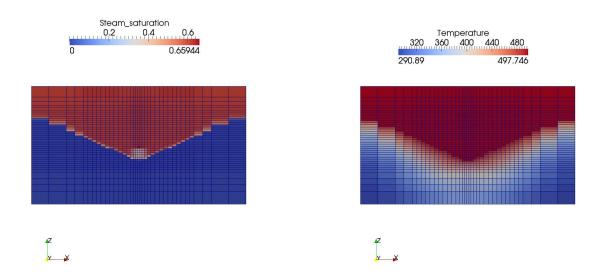
Figure 4.8: steam saturation (left) and temperature of the reservoir (right) at 4000 days.
