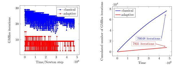
Figure 2.30: GMRes iterations at each time and Newton step (left) and cumulated number of GMRes iterations as a function of time (right) for the test case of Section 2.5.4.1. Average number of GMRes iterations per time and Newton iteration step: 27 iterations (classical), 6 iterations (adaptive). Average number of GMRes iterations per time step: 104 iterations (classical), 9 iterations (adaptive)
