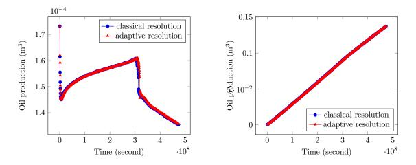
Figure 2.24: Rate (left) and cumulated rate (right) of oil production during the simulation, classical resolution vs. adaptive resolution for the test case of Section 2.5.4.1
