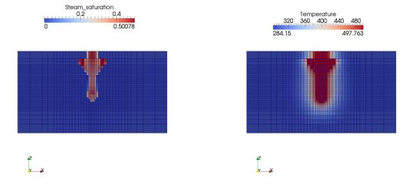
Figure 4.6: Forming the steam chamber: steam saturation (left) and temperature of the reservoir (right) at 600 days.
