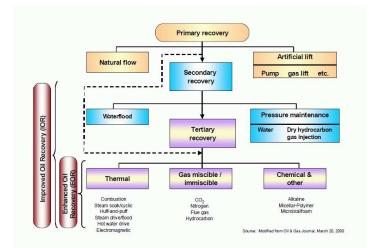
Figure 1: Classification of hydrocarbon recovery methods.
