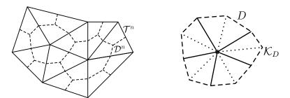
Figure 1.2: Simplicial mesh  $\mathcal{T}^n$  and the associated vertex-centered dual mesh  $\mathcal{D}^n$  (left) and the fine simplicial mesh  $\mathcal{K}_D$  of  $D \in \mathcal{D}^n$  (right)
