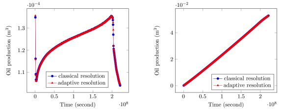
Figure 2.3: Rate (left) and cumulated rate (right) of oil production during the simulation, classical resolution vs. adaptive resolution for the test case of Section 2.5.2
