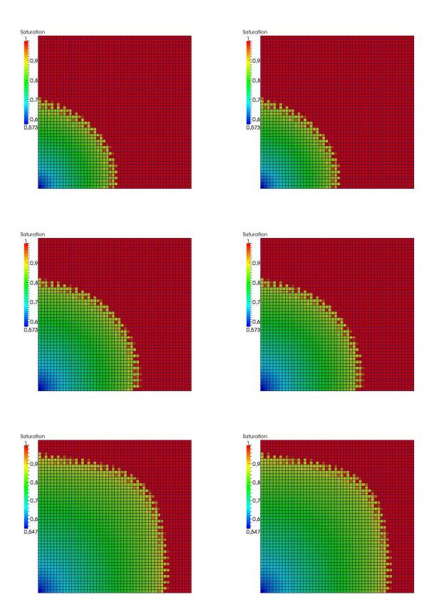
Figure 2.11: Liquid saturation, classical (left) and adaptive (right) resolutions at times 30 months, 50 months, and 84 months for the test case of Section 2.5.3.1
