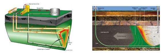
Figure 4: Vapex (left) and Thai (right) process.
