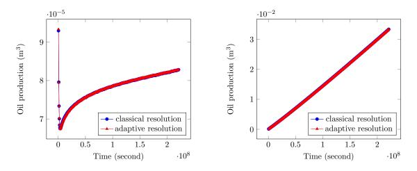
Figure 2.10: Rate (left) and cumulated rate (right) of oil production during the simulation, classical resolution vs. adaptive resolution for the test case of Section 2.5.3.1
