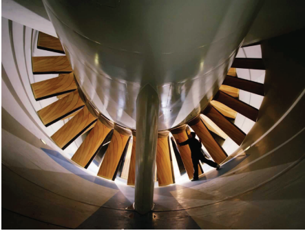
Figure 4.9: Grady McCoy stands in the Langley Research Center’s 16 foot transonic wind tunnel in 1990. Before the tunnel was mothballed in 2004 it supported most major military programs both in their development stage and ongoing propulsion integration research including all fighters since 1960 (F-14, F-15, F-16, F-18 and the Joint Strike Fighter) (source: NASA). Such facilities were used for the design and test of new technologies dedicated to enhance sport performance.
