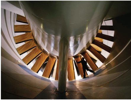
Figure 4.9: Grady McCoy stands in the Langley Research Center's 16 foot transonic wind tunnel in 1990. Before the tunnel was mothballed in 2004 it supported most major military programs both in their development stage and ongoing propulsion integration research including all fighters since 1960 (F-14, F-15, F-16, F-18 and the Joint Strike Fighter) (source: NASA). Such facilities were used for the design and test of new technologies dedicated to enhance sport performance.
