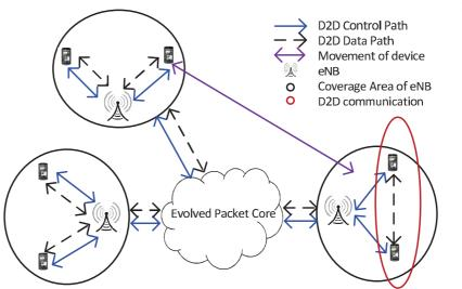
Figure 5.2: D2D communication diagram.
