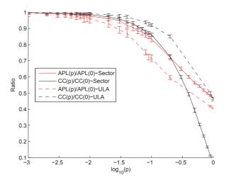
Figure 3.1: Effect of beamforming on the APL and the CC when the nodes are using different antenna models.
