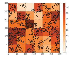
Figure 2.7: Deployment and the node density per  $50*50m^2$  region after applying the Thinning process on the deployment as shown by Fig. 2.6 with  $r_b = 15$  and  $N_{min} = 6$ . The density is shown by the color-bar.
