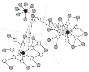
(b) Three unconnected components with three regions when g = 4. Here, the node x can create the beam either towards y or z, but because the *hopcount* to y and z is same as  $\infty$ , x randomly decides between y and z to connect to.
