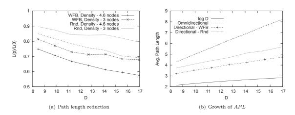
Figure A.3: Path length reduction by beamforming at nodes with high values of WFB.
