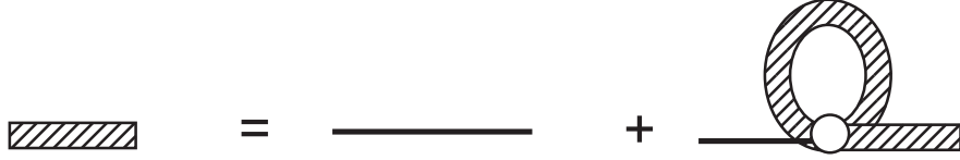
Figure 2.3. Diagrammatic form of the Dyson-type equation. This equation is specific for the partition function of an individual chain g_n with cactus-like topology (2.19).
