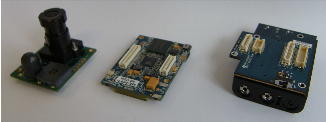
FIGURE 7.1: Multimedia board - Imote2 processor board - Battery board
