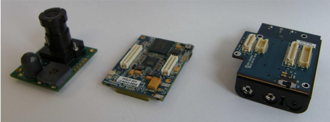
FIGURE 7.1: Multimedia board - Imote2 processor board - Battery board
