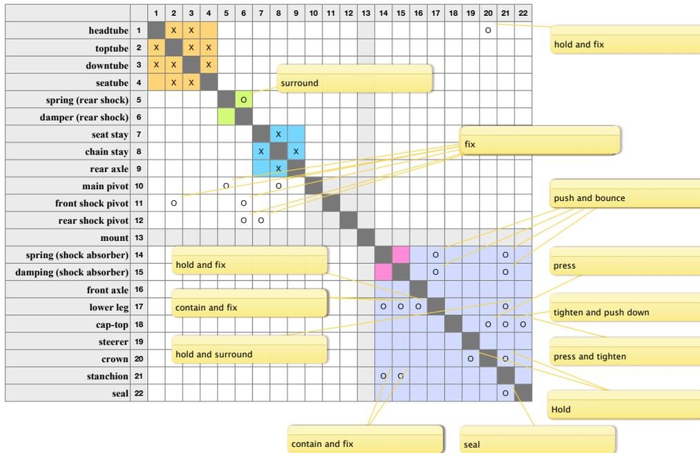
FIGURE 6.6 – Component-base DSM
