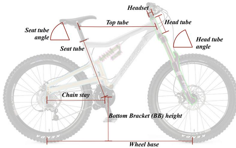
FIGURE B.10 – Frameset geometry
