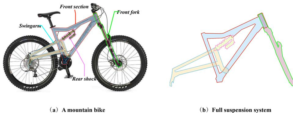
FIGURE 6.2 – The full suspension system for mountain bike
