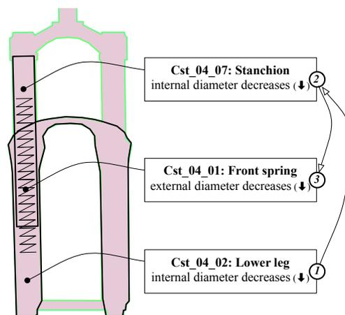
FIGURE 6.7 – Change propagation between multiple constructs
