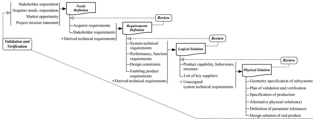
FIGURE 6.4 – Evolution model of full suspension system
