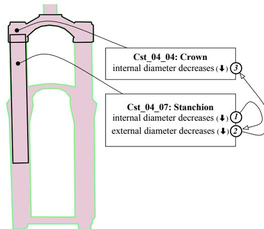
FIGURE 6.8 – Change propagation within one construct
