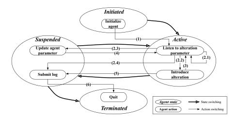
FIGURE 5.16 – Life cycle of ChangeGenerator
