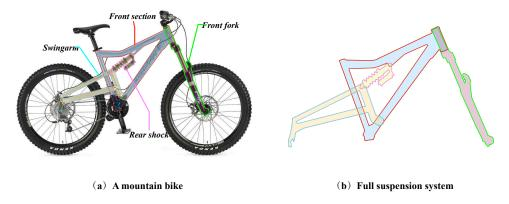
FIGURE 6.2 – The full suspension system for mountain bike
