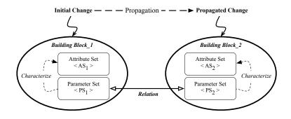
FIGURE 4.4 – Change propagation conceptual model
