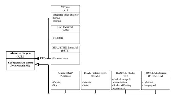
FIGURE B.11 – Supply chain of A.B.
