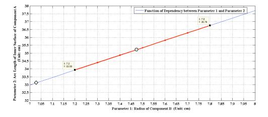
FIGURE 4.7 – Dependency between Radius of Component B (i.e., Parameter 1) and Arc length of inner surface of Component A (i.e., Parameter 2)
