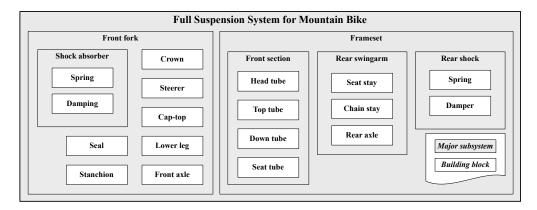
FIGURE 6.5 – Architecture of full suspension system
