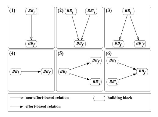
FIGURE 4.14 – Effort-based change propagation patterns (1, 2, 3) and non-effort-based change propagation patterns (4, 5, 6)
