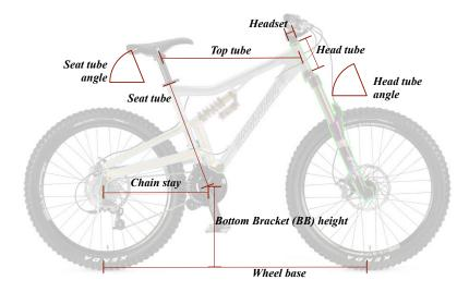
FIGURE B.10 – Frameset geometry
