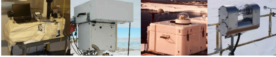
Figure 6.1: Images of the the Dobson spectrometer at South Pole (image courtesy: http://www.esrl.noaa.gov/gmd/ozwv/dobson/ ), the Brewer spectrometer at Zhongshan (image courtesy: http://www.theozonehole.com/ ), the SAOZ instrument at Dumont d'Urville (image courtesy: F. Goutail, CNRS, Paris) and the DOAS instrument at Neumayer (image courtesy: http://www.awi.de/typo3temp/pics/ ) in Antarctica.
