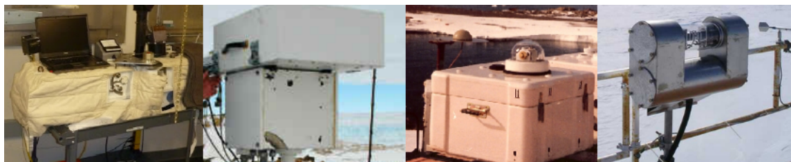
Figure 6.1: Images of the the Dobson spectrometer at South Pole (image courtesy: http://www.esrl.noaa.gov/gmd/ozwv/dobson/ ), the Brewer spectrometer at Zhongshan (image courtesy: http://www.theozonhole.com/ ), the SAOZ instrument at Dumont d'Urville (image courtesy: F. Goutail, CNRS, Paris) and the DOAS instrument at Neumayer (image courtesy: http://www.awi.de/typo3temp/pics/ ) in Antarctica.
