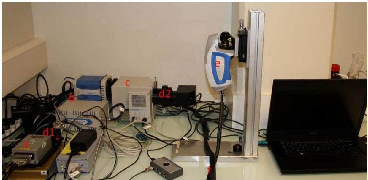
FIGURE 12: SYSTEME MICRO-SONDE RAMAN: (A) SOURCE LASER, (B) CHARGED COUPLED DEVICE (CCD), (C) MICRO HR, (D1 ET D2) SHUTTER LASER ET SHUTTER SPECTROMETRE RESPECTIVEMENT, (F) FIBRE PERMETTANT UNE CONFOCALITE DE 5  $\mu\text{m}$  ET (E) MICRO-SONDE CONFocale
