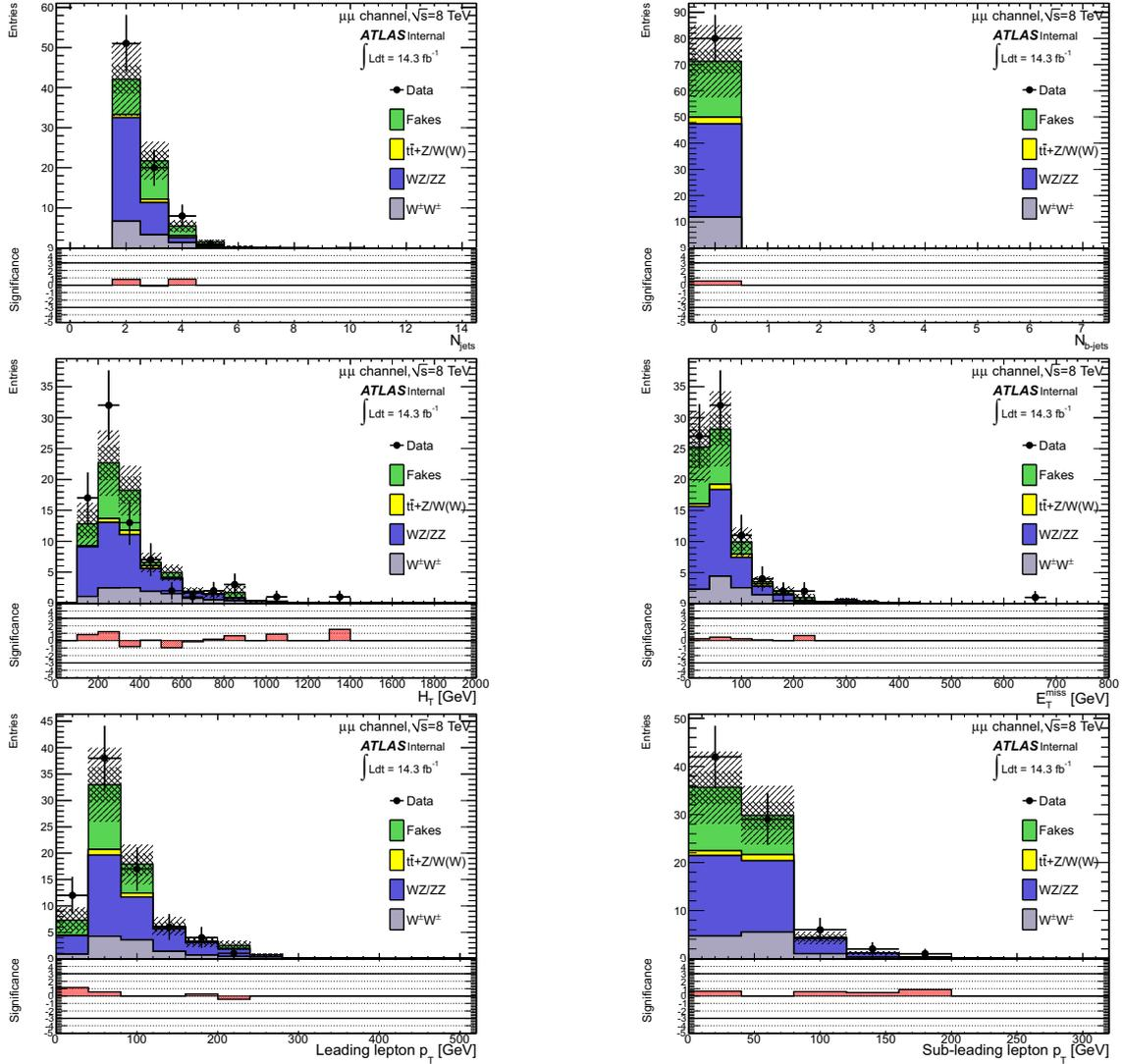
**Figure 7.31:** Distributions of some kinematic variables in the  $\mu\mu$  channel, after the zero- $b$ -tag control region selection at 8 TeV, for both the background estimation and the data. The bottom plots show the significance of the measured number of events in the data compared to the estimated number of events from the backgrounds.
