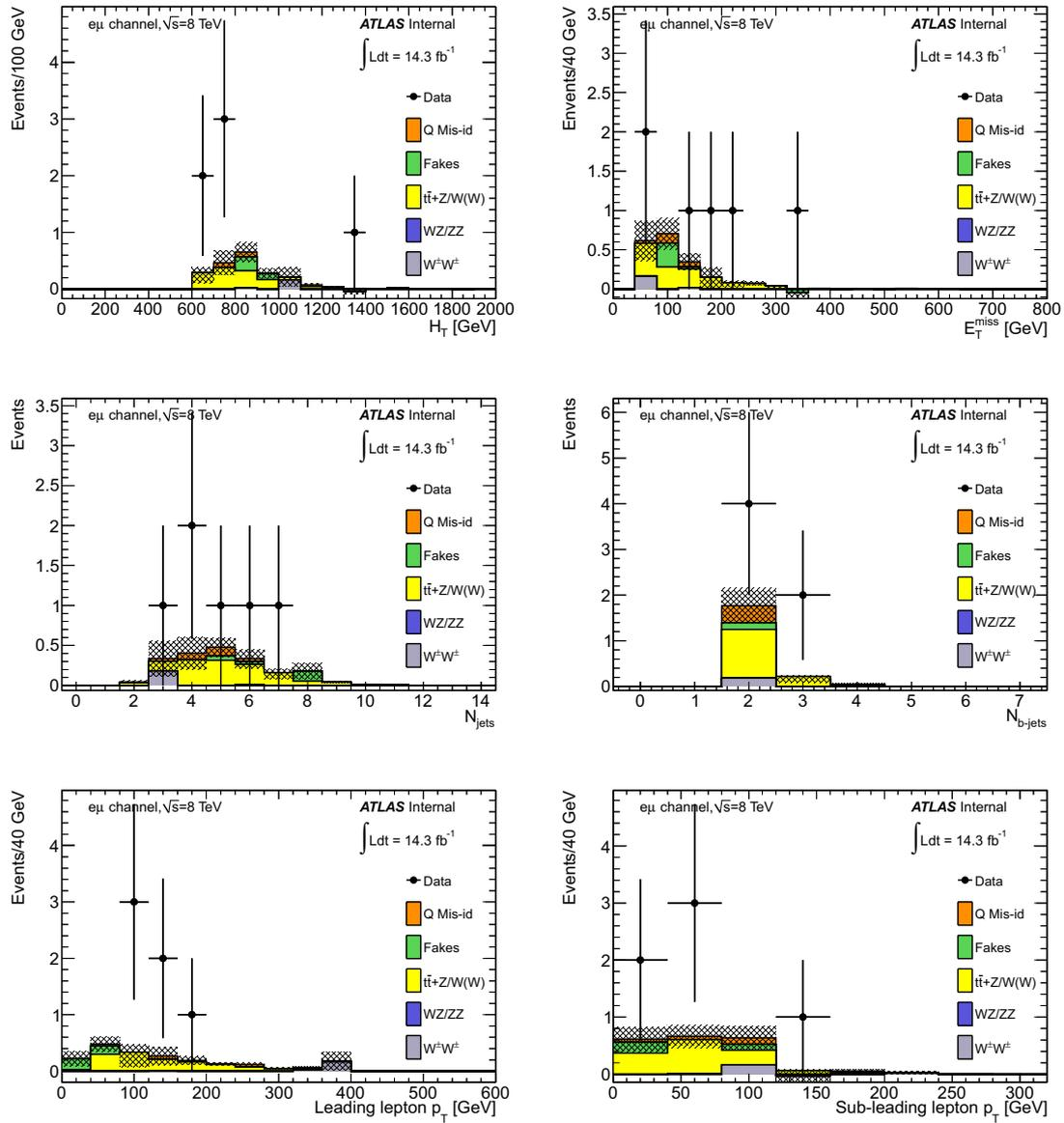
**Figure C.5:** Distribution of some kinematical variables for the data (points) and for the estimated background (histogram), after applying the final selection in the  $e\mu$  channel at  $\sqrt{s} = 8$  TeV. The internal shaded areas correspond to the statistical uncertainties on the background while the external shaded areas correspond to the total uncertainties. For the Monte Carlo samples, systematic uncertainties include only the production cross section uncertainties.
