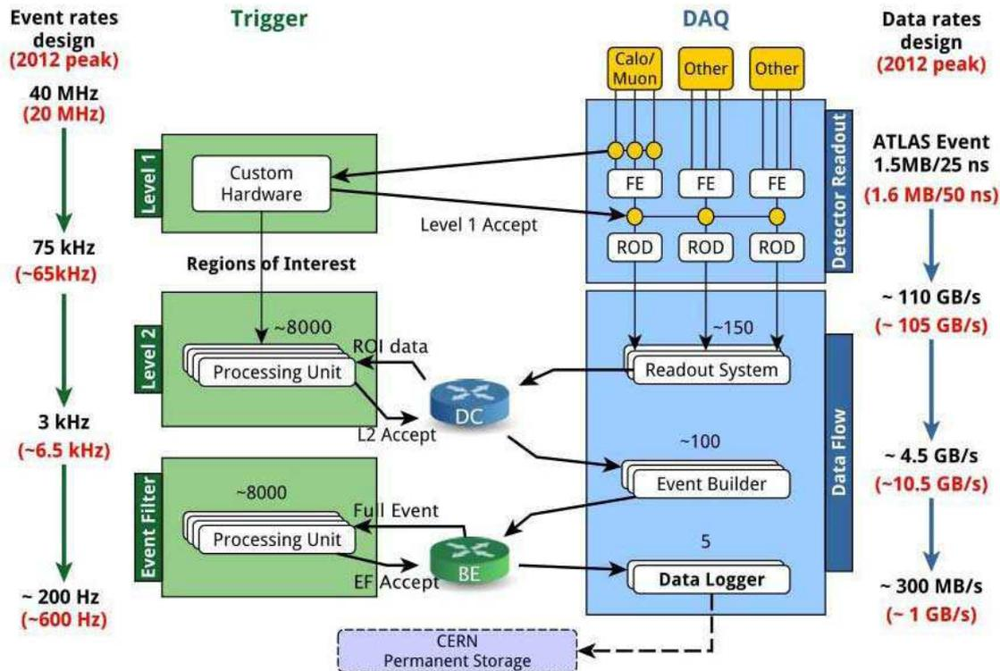
Figure 3.18: ATLAS trigger and data acquisition system [118].
