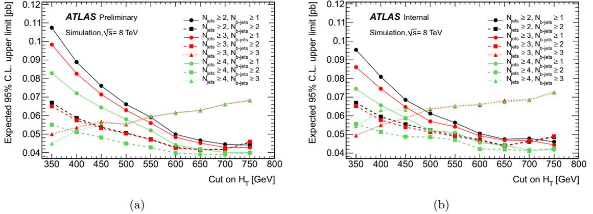
**Figure 8.2:** Expected 95% C.L. upper limit on the four tops contact interaction production cross-section as a function of the cut on  $H_T$  for various sets of cuts on the number of jets (different colors) and  $b$ -jets (different markers), using a cut on the  $E_T^{\text{miss}} > 40$  GeV (a) and  $E_T^{\text{miss}} > 60$  GeV (b) for the analysis done at  $\sqrt{s} = 8$  TeV. The final selection is chosen so that it can provide the minimum value on the cross-section.
