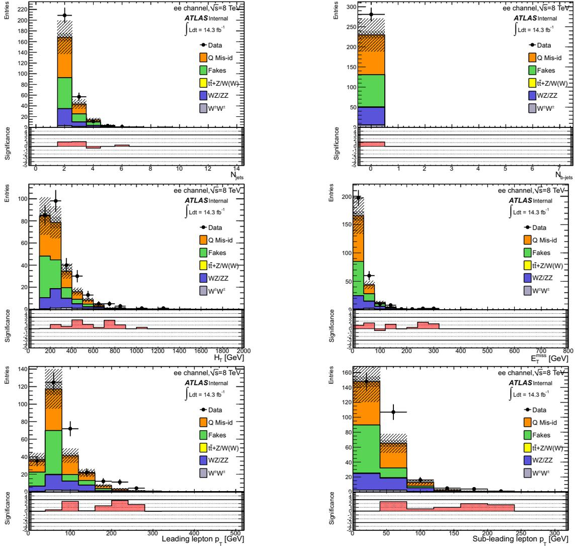
**Figure 7.29:** Distributions of some kinematic variables in the  $ee$  channel, after the zero- $b$ -tag control region selection at 8 TeV, for both the background estimation and the data. The bottom plots show the significance of the measured number of events in the data compared to the estimated number of events from the backgrounds.
