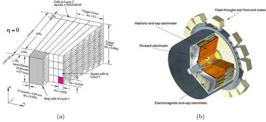
**Figure 3.8:** a) One example of a barrel module of the EM calorimeter showing its three different layers, the granularity in  $\eta$  and  $\phi$  of the cells of each of the three layers, the trigger towers, and its accordion structure. b) Cut-away view of an endcap cryostat showing the positions of the three endcap calorimeters [4].
