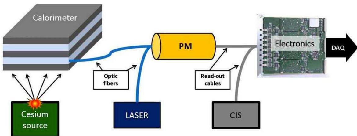
Figure 4.1: Hardware calibration chain of ATLAS TileCal.
