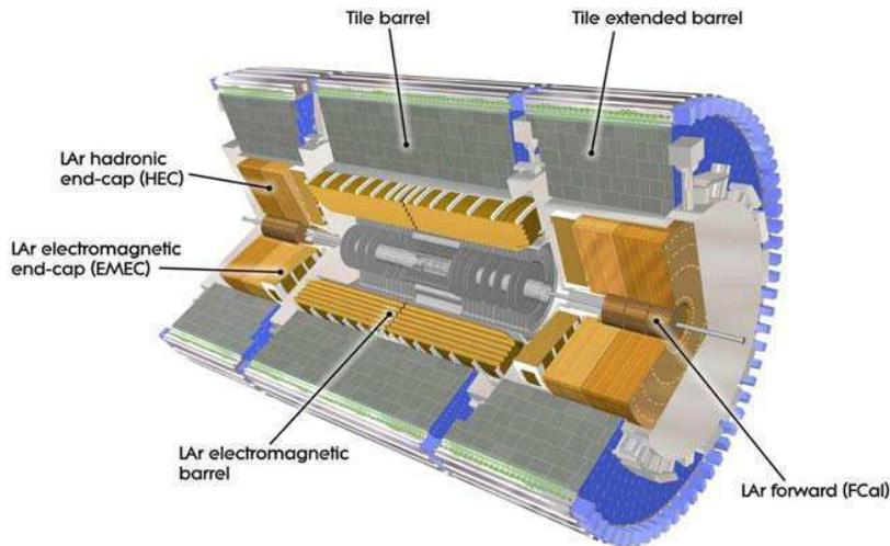
**Figure 3.7:** Cut-away view of the ATLAS calorimeter system. Calorimeters with LAr as active medium are situated in the inner section, while in the outer section the sampling medium consists of scintillator tiles [4].
