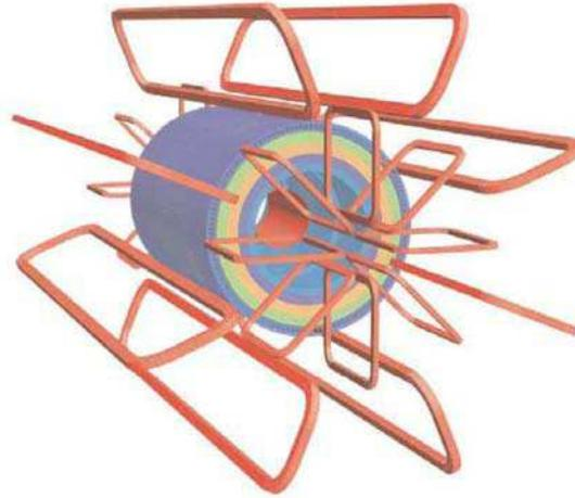
**Figure 3.17:** Geometry of magnet windings and Tile calorimeter steel. The solenoid magnet lies inside the calorimeter system. The eight barrel toroid coils interleaved with the endcap coils are also visible.
