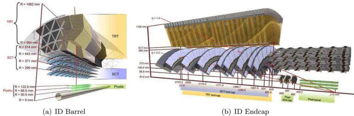
**Figure 3.3:** The barrel (a) and endcap (b) tracking system of the ATLAS inner detector. The barrels of each sub-detector are arrayed in concentric cylinders around the beam line, while the endcaps are mounted on disks perpendicular to it.
