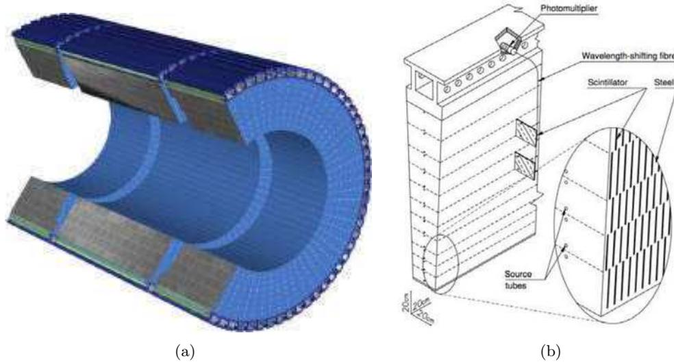
**Figure 3.9:** a) Cut-away view of the Tile calorimeter. b) Structure of a module of the Tile calorimeter, showing the placement of the scintillator tiles, the steel plates and the readout components [4].
