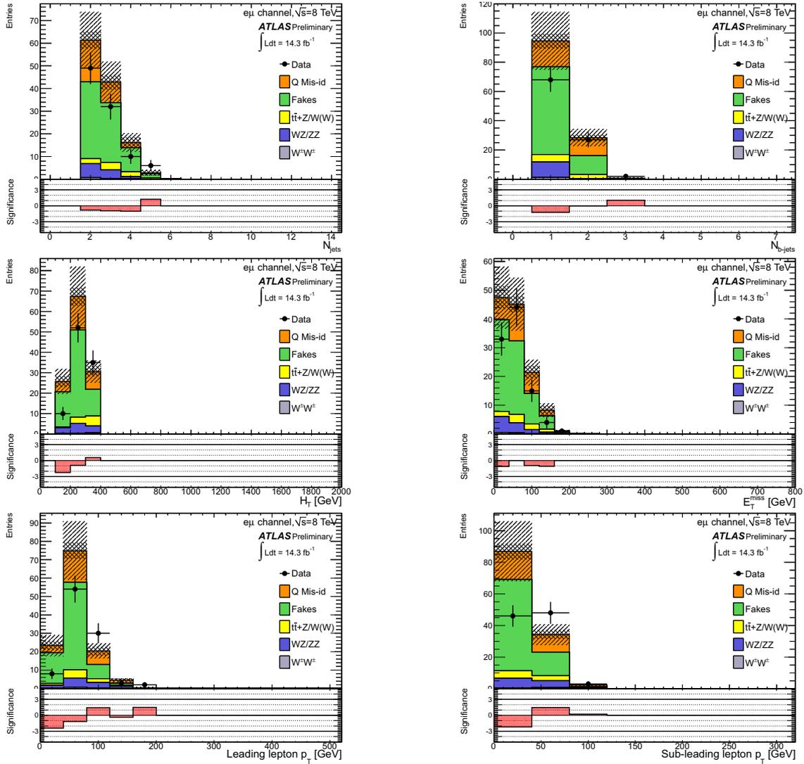
**Figure 7.24:** Distributions of some kinematical variables in the  $e\mu$  channel, after the  $E_T^{\text{miss}}$  control region selection at 8 TeV, for both the background estimation and the data. The bottom plots show the significance of the measured number of events in the data compared to the estimated number of events from the backgrounds.
