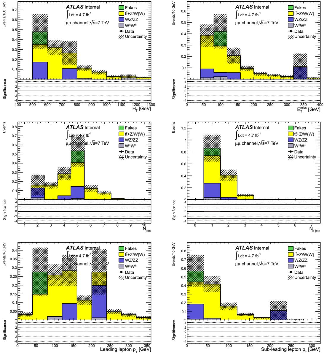
**Figure C.3:** Distribution of some kinematical variables for the data (points) and for the estimated background (histogram), after applying the final selection in the  $\mu\mu$  channel at  $\sqrt{s} = 7$  TeV. The internal shaded areas correspond to the statistical uncertainties on the background while the external shaded areas correspond to the total uncertainties. For the Monte Carlo samples, systematic uncertainties include only the production cross section uncertainties.
