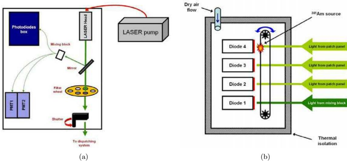
**Figure 4.2:** The LASER box (a) contains the light source and the internal calibration system. The photodiodes used to measure the intensity of the laser light are located inside the photodiodes box (b).
